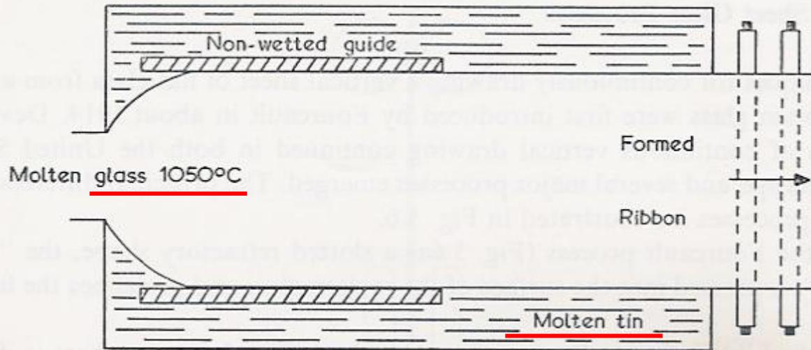
4. Manufacture of thick float ribbon (~ 10 – 25 mm)
