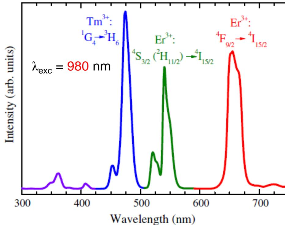
Simultaneous up-conversion emission of the three primary colours (blue, green and red) under infrared excitation at 980 nm with a power up to 200 mW of 94.5 SiO<sub>2</sub>-5 LaF<sub>3</sub> tri-doped with 0.3 mol% Yb<sup>3+</sup>, 0.1 mol% Er<sup>3+</sup> and 0.1 mol% Tm<sup>3+</sup> sol-gel derived nano-glass-ceramics (SOL-YET). Assignment of emission bands with corresponding transitions of rare-earth ions is indicated
