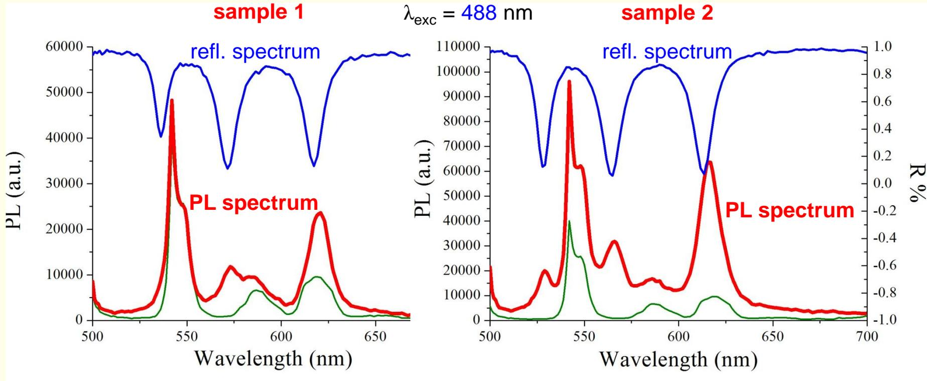
The **three** distinct PL peaks of  $\text{Tb}^{3+}$  ions were **broadened** to combine into a **continuous fluorescence band**.
