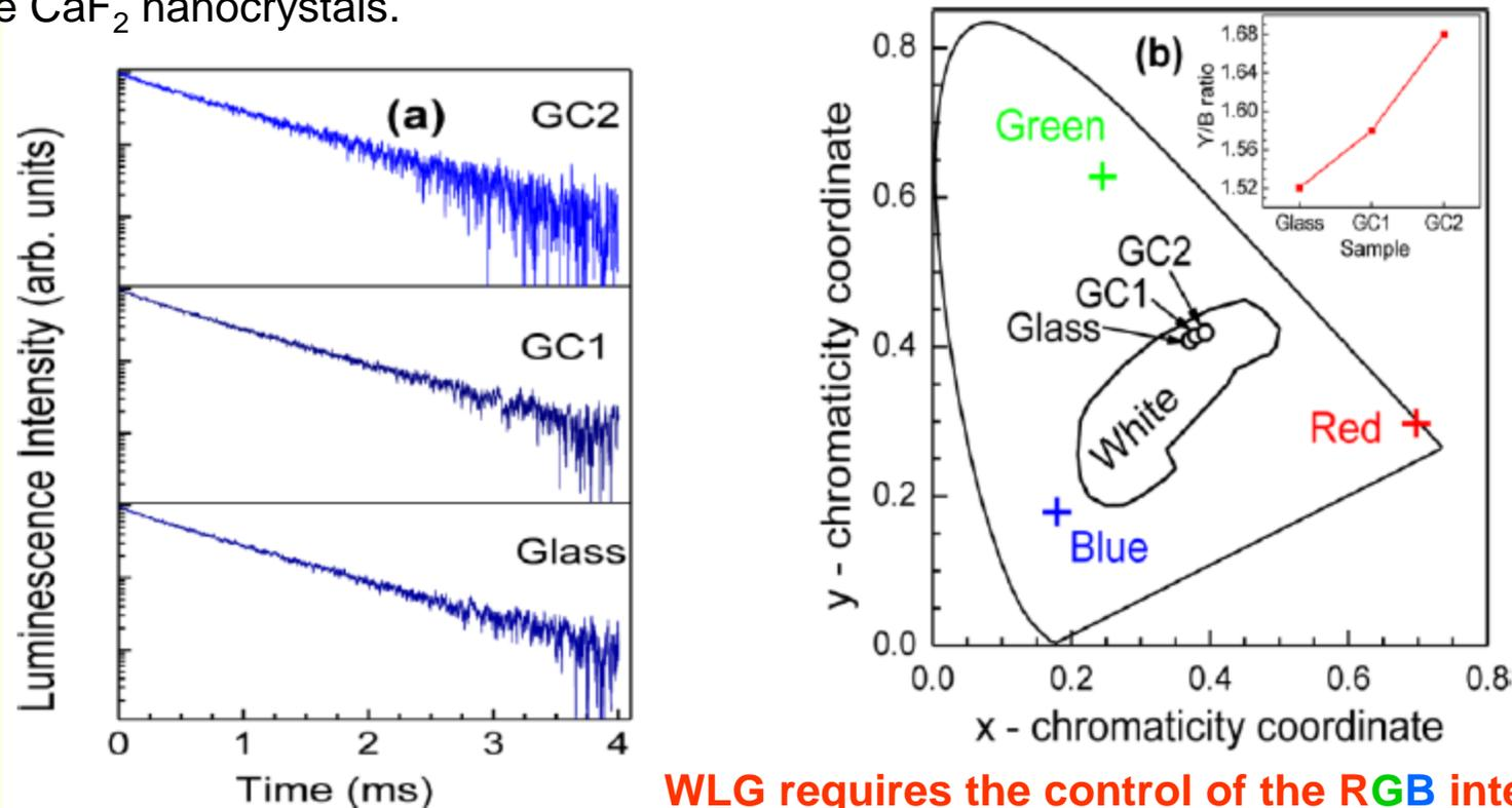
(a) Luminescence decay curves of 0.1 mol % of Dy<sup>3+</sup>:glass, GC1 and GC2 and (b) The CIE-1931 chromaticity color diagram showing the white light emission from the 0.1 mol % of Dy<sup>3+</sup>:glass, GC1 and GC2. Inset shows the variation of Y/B with heat treatment temperature.
