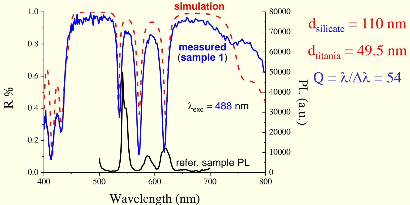
The profile of the measured reflection spectrum coincided very well with the theoretical curve, including the stop band, the defect peaks and the fringes.
