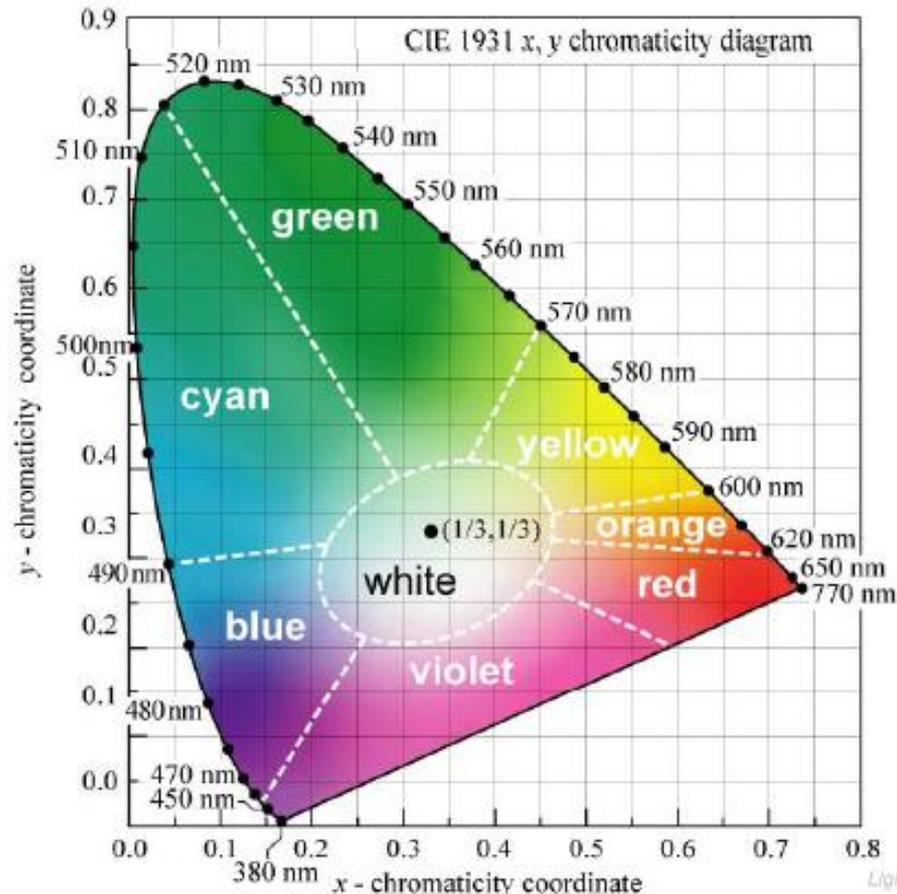
CIE 1931 (x, y) chromaticity diagram. Mono-chromatic colors are located on the perimeter. Color saturation decreases towards the center of the diagram. White light is located in the center. Also shown are the regions of distinct colors. The equal-energy point is located at the center and has the coordinates  $(x, y) = (1/3, 1/3)$ .
