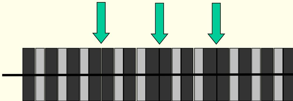
Triple coupled microcavity
