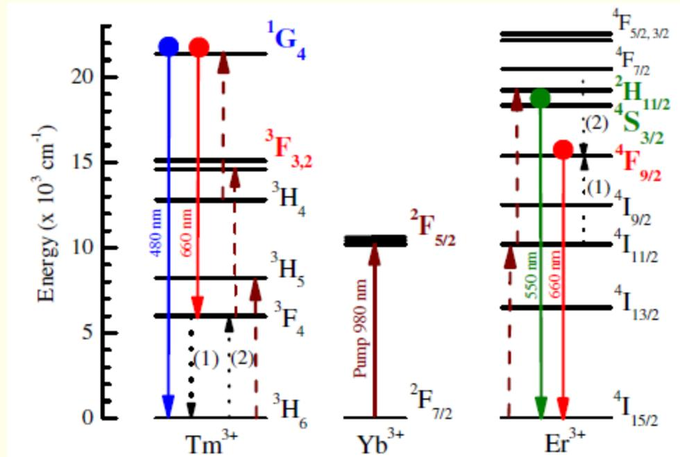
Energy level diagram of the  $\text{Er}^{3+}$ ,  $\text{Yb}^{3+}$  and  $\text{Tm}^{3+}$  copopants. Solid arrows indicate pump and up-conversion emission transitions. Dash lines indicate 2- and 3-photon up-conversion processes. Dot lines labelled with (1) and (2) indicate energy transfer processes among  $\text{Er}^{3+}$  and  $\text{Tm}^{3+}$  ions responsible of the enhancement of the red emission
