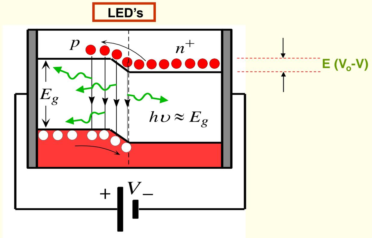
A **LED** is a **p-n junction diode** made from a **direct bandgap SC**, e.g. GaAs, in which **electron-hole pair (EHP) recombination** results in **emission of a photon** of energy  $h\nu \sim E_G$ .
