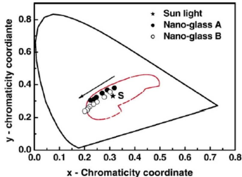
The position of white light emission from nano-glasses in the chromaticity diagram (CIE 1931) recorded at different pump powers. The area inside the dashed line shows the white light region, and the arrow indicates an increase in the pump power .
