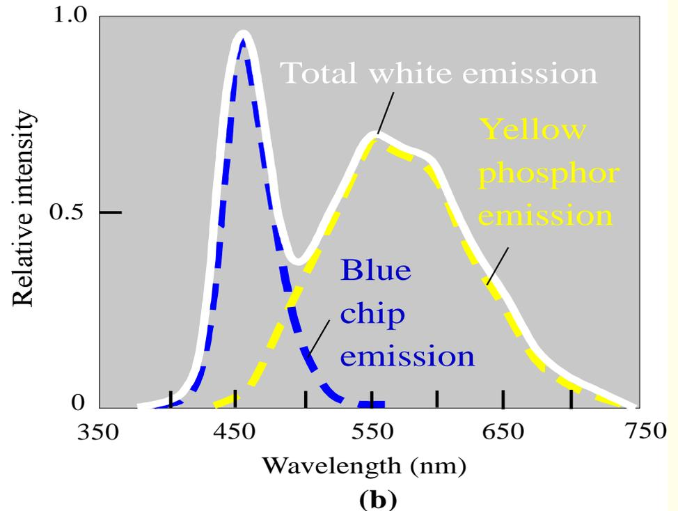
(a) A typical “white” LED structure. (b) The spectral distribution of light emitted by a white LED. Blue luminescence is emitted by the GaInN chip and “yellow” phosphorescence or luminescence is produced by a phosphor. The combined spectrum looks “white”.
