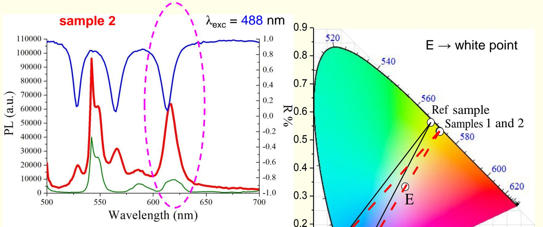
**White light** can almost be obtained by mixing the modified PL with the blue exciting light, while this is **impossible** for the PL of the **reference sample**.
