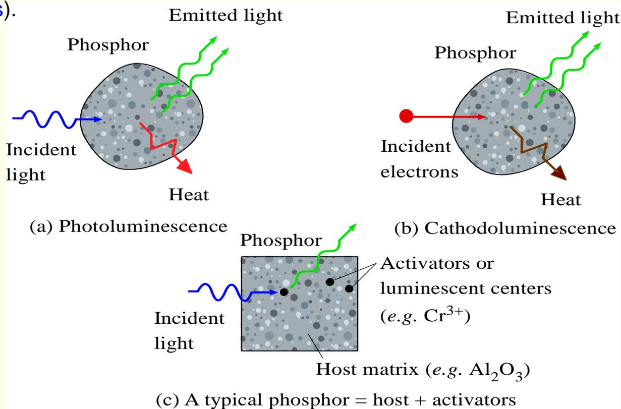
Photoluminescence, cathodoluminescence and a typical phosphor
