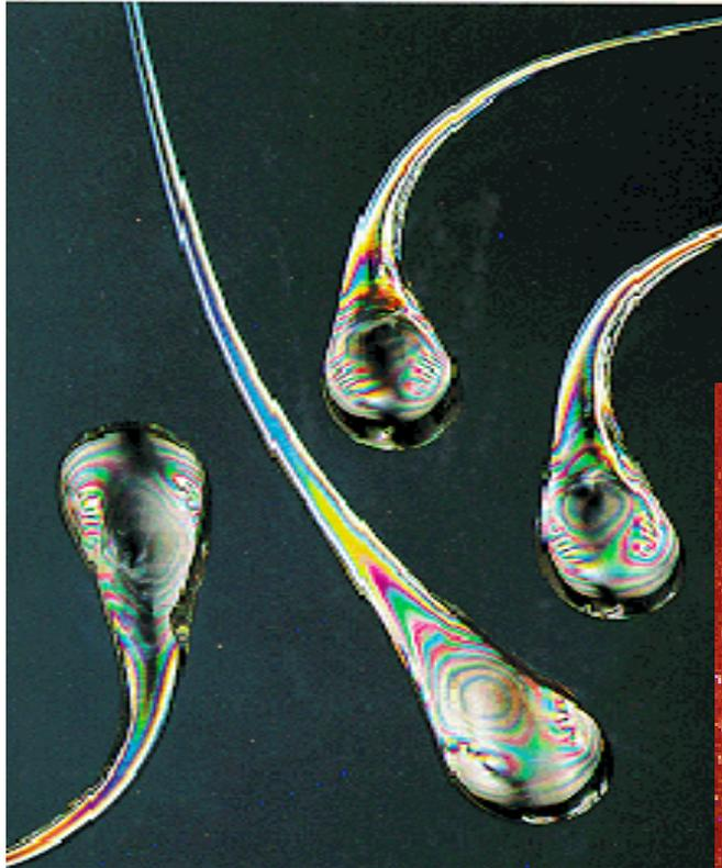
***Formation-induced attributes dictate the form, performance and lifetime on a resulting glass part. Here, residual stress frozen into a Prince Rupert's drop during its formation (which appears as birefringence under crossed polarizers) ultimately limits the drop's mechanical stability and life.***
