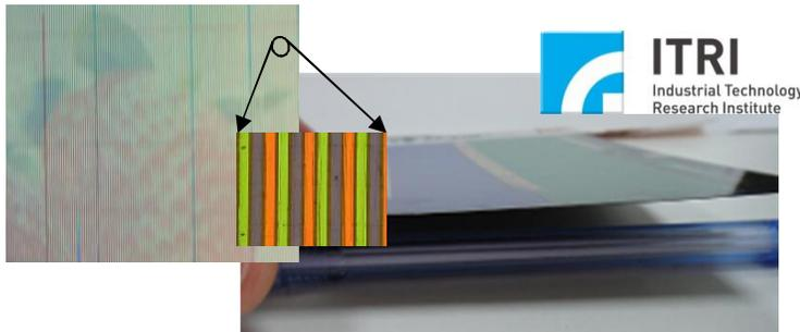
Color ChLCD, 5" diag.,  $<210\mu\text{m}$  thick, 80ppi
