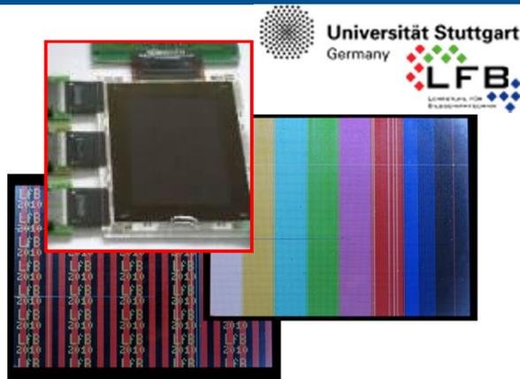
Color LCD, 4" diag.,  $<170\mu\text{m}$  thick, qVGA
