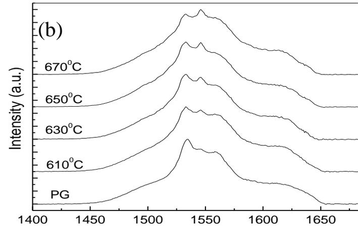
(a) Upconversion emission, and (b) near-infrared emission spectra of glass ceramics under 980 nm excitation
