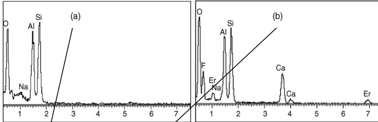
EDS spectra with nano-sized probe from: (a) glass matrix, and (b) an individual nanocrystal, of 2 mol% Er doped glass ceramic
