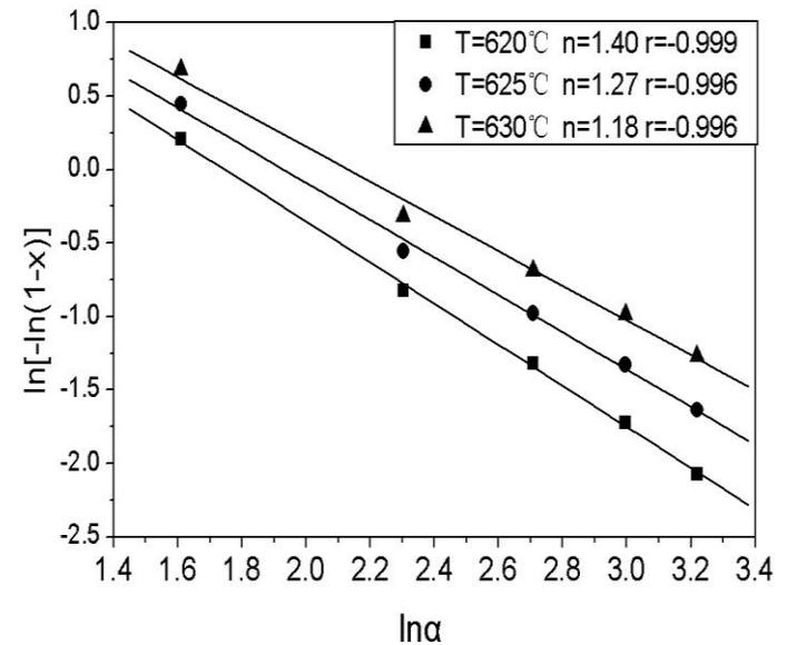
**Example illustrating the determination of  $E_a$  and  $n$  for crystallization in glass matrix**
