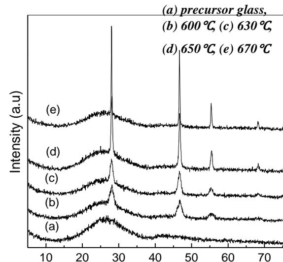
Heating induced precipitation of CaF<sub>2</sub> nanocrystals
