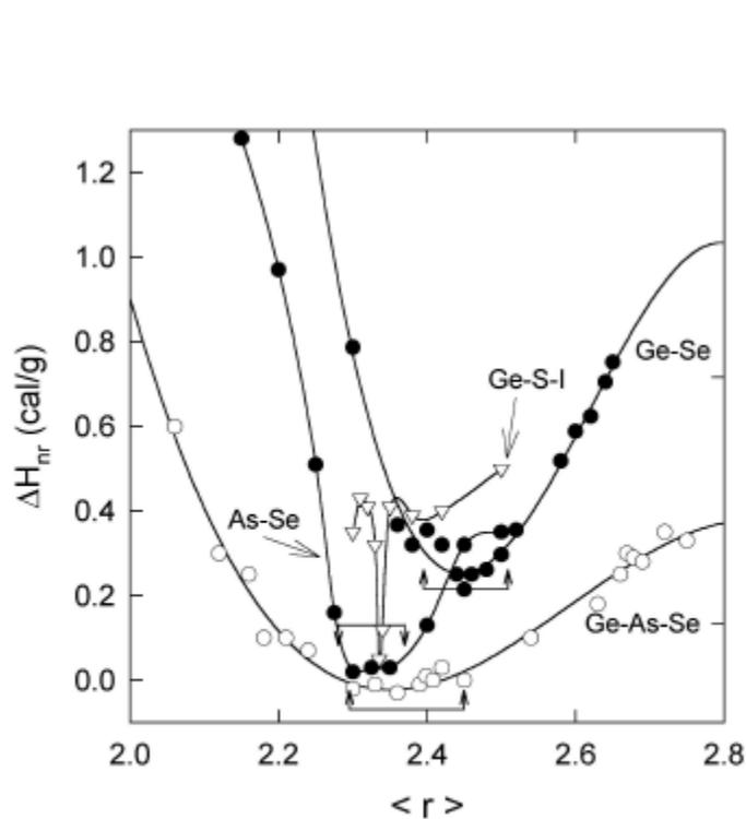
Fig. 4. Non-reversing heat,  $\Delta H_{nr}$ , as a function of mean coordination number  $\langle r \rangle$  for four different glass systems. The Ge-As-Se ternary shows the widest window (Ref. 5) while the Ge-S-I the narrowest (Ref. 7).
