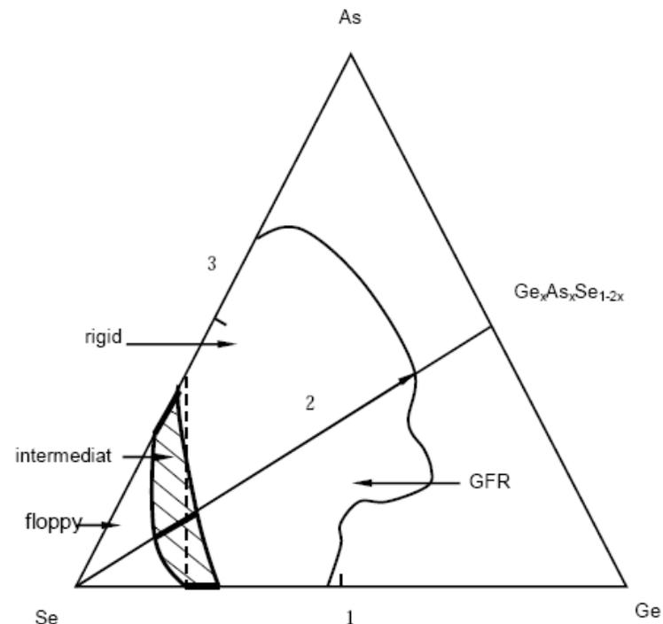
Fig. 5. The glass-forming region in the Ge-As-Se ternary glass system. The broken line corresponds to  $\langle r \rangle = 2.40$ . The shaded region gives the opening of the intermediate phase between the floppy and the rigid phases, and it straddles the  $\langle r \rangle = 2.40$  line.
