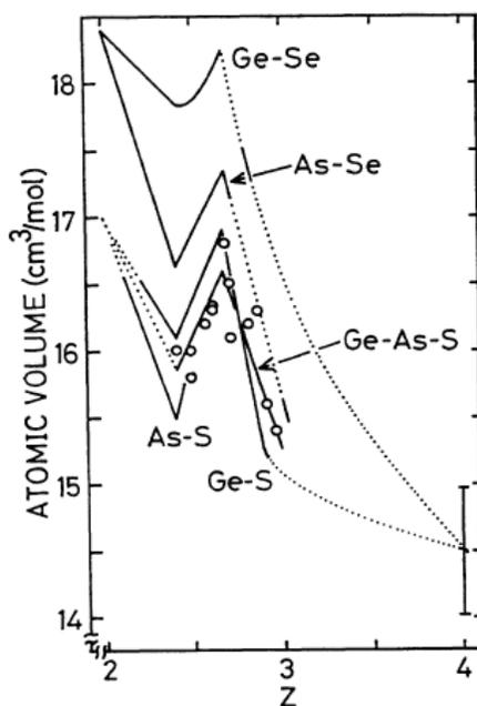
FIG. 2. The atomic volumes for various chalcogenide glasses as a function of the average coordination number  $Z$ . The present results for Ge-As-S glasses are plotted by circles. Solid lines for binary alloys show representative tendencies with an accuracy of  $\pm 0.1 \text{ cm}^3/\text{mol}$ . Dotted lines depict estimated behaviors.
