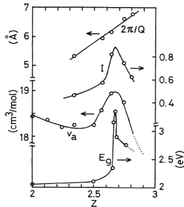
FIG. 10. The atomic volume  $v_a$ , the optical band-gap energy  $E_g$ , the FSDP position  $2\pi/Q$ , and the normalized FSDP intensity  $I$  for Si-Se glasses as a function of the average coordination number  $Z$ .
