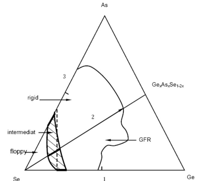
Fig. 5. The glass-forming region in the Ge-As-Se ternary glass system. The broken line corresponds to  $\langle r \rangle = 2.40$ . The shaded region gives the opening of the intermediate phase between the floppy and the rigid phases, and it straddles the  $\langle r \rangle = 2.40$  line.
