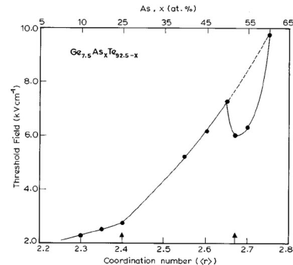
FIG. 2. Composition dependence of the electrical switching fields ( $E_t$ ) of  $\text{Ge}_{7.5}\text{As}_x\text{Te}_{92.5-x}$  glasses. The vertical arrows at  $\langle r \rangle = 2.4$  and  $2.67$  indicate the mechanical and chemical thresholds, respectively.
