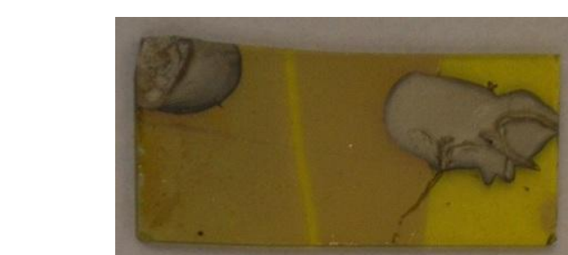
Typical sample – gap between Au pads
