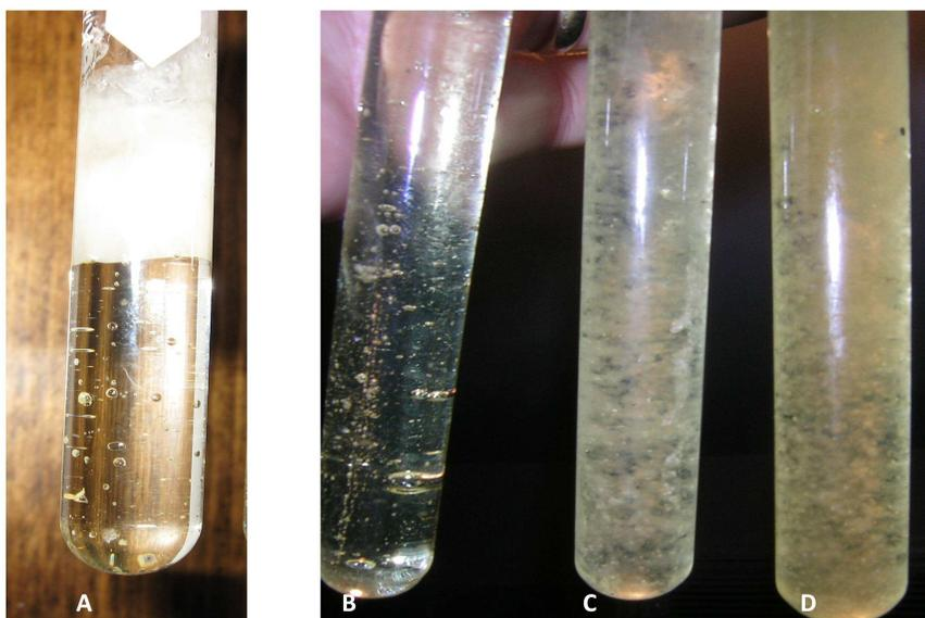
Figure 7. (A) Growth of crystals at the surface (top) of sugar glass in test tube at room temperature after several weeks of high humidity. The photo on the right shows the progression of bulk crystallization from an unheated clear candy glass (B), to one that is heated in a home oven set to 250° F (120°C) for approximately 20 minutes (C & D).
