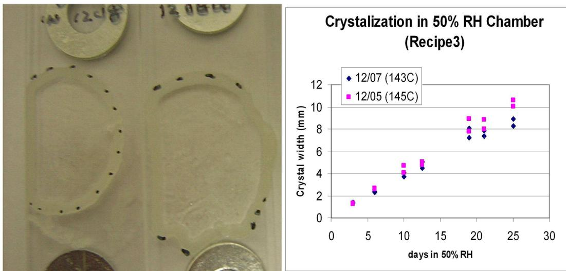
Figure 8. Photograph of crystal growth on outer edge of two samples taken on day 5 after placing in the 50% RH chamber. Note the uniform thickness of the crystal layer in both samples. On right, data show increasing width of crystal layer with time for a standard recipe glass. Two different batches are included (diamonds and squares). Note that the  $145^\circ\text{C}$  sample (squares) also includes a replicate.
