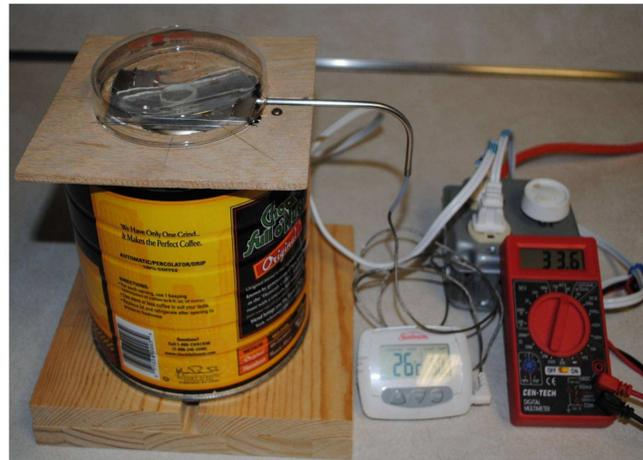
Figure 9. Sketch of the light bulb sample oven for the crystallization vs. temperature studies. (Right) Photograph of the complete apparatus with dimmer control, digital thermometer and digital volt meter (DVM) for monitoring voltage across light bulb heating element.
