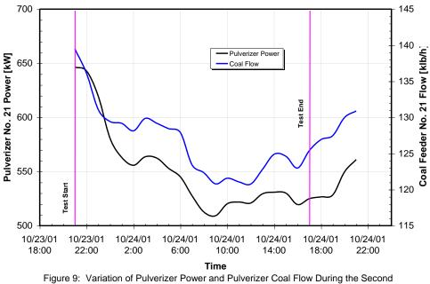
Figure 9: Variation of Pulverizer Power and Pulverizer Coal Flow During the Secon Coal Burn Test for No. 21 Pulverizer
