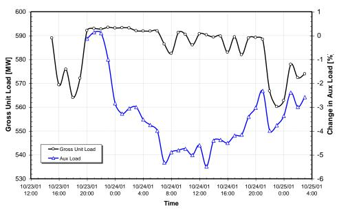
Figure 10: Reduction in Auxiliary Power Measured During the Second Coal Burn Test
