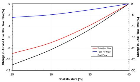
Figure 1: Effect of Coal Moisture on Flow Rates of Air, Flue Gas and Coal
