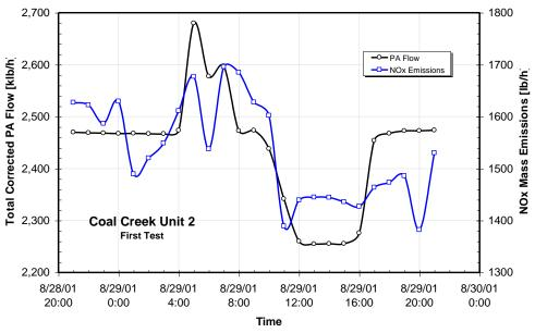
Figure 13: Variation in PA Flow and Mass Emissions of NO<sub>x</sub> During the First Coal Burn Test
