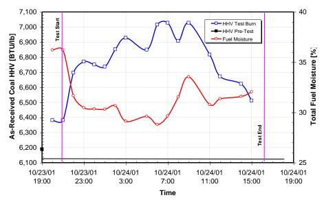
Figure 6: Variation of Coal HHV and Moisture Content During the Second Coal Burn Test
