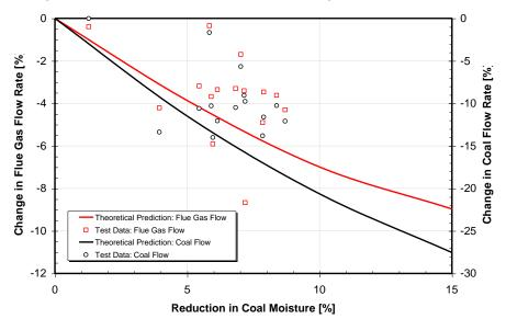
Figure 8: Change in Coal and Flue Gas Flow Rates with Coal Moisture
