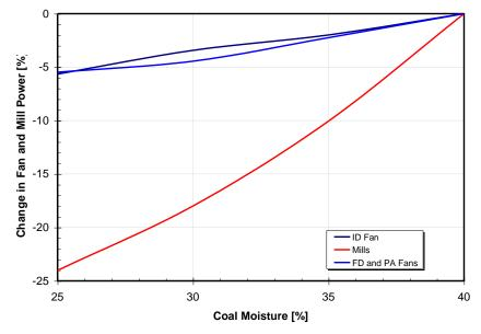
Figure 2: Effect of Coal Moisture on Fan Power
