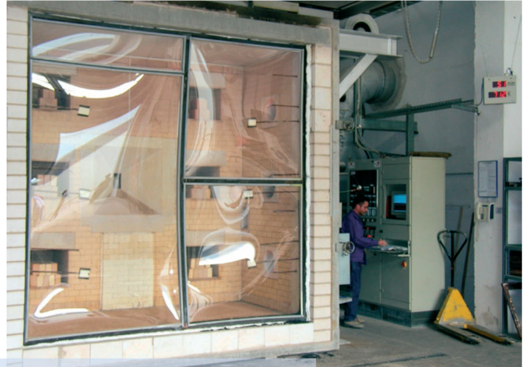
Even in simple frame constructions borosilicate glass resists high temperatures and has long staying power.
