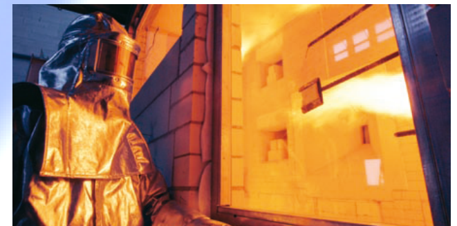
Even in simple frame constructions borosilicate glass resists high temperatures and has long staying power.
