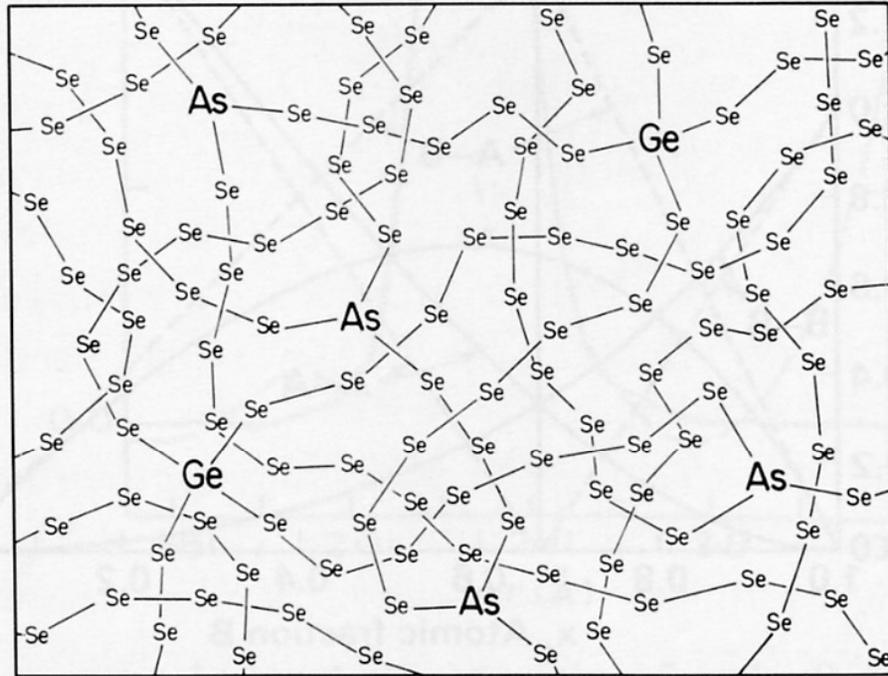
2-D representation of the bonding in Ge-As-Se glass. Note cross-linking of linear chains by As (3-coordination) and Ge (4-coordination). (After R. Zallen, *The Physics of Amorphous Solids*, Fig. 3.7, p. 98. Wiley & Sons, New York, 1983. Reproduced with permission of the publishers.)
