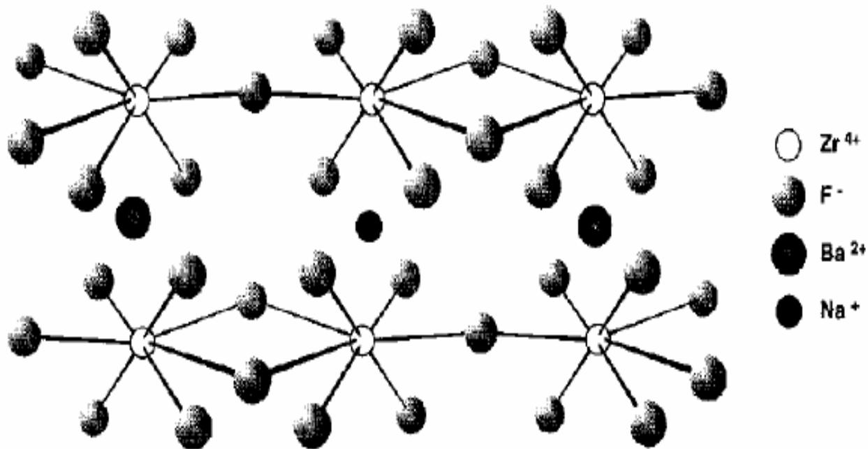
Chain-like skeleton in the structure of a  $\text{ZBLAN}_{66}$  glass (57.0  $\text{ZrF}_4$ -28.1  $\text{BaF}_2$ -3.3  $\text{LaF}_3$ -5.0  $\text{AlF}_3$ -6.6  $\text{NaF}$ , in mol%).
