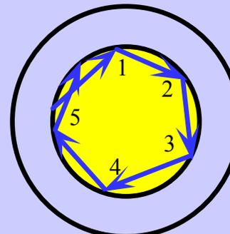
(b) A skew ray does not have to cross the fiber axis. It zigzags around the fiber axis.
