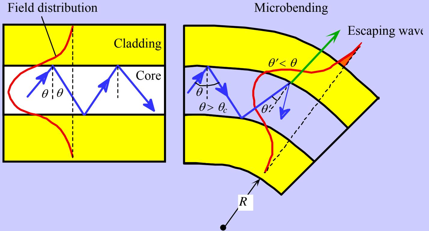
Sharp bends change the local waveguide geometry that can lead to waves escaping. The zigzagging ray suddenly finds itself with an incidence angle  $\theta'$  that gives rise to either a transmitted wave, or to a greater cladding penetration; the field reaches the outside medium and some light energy is lost.
