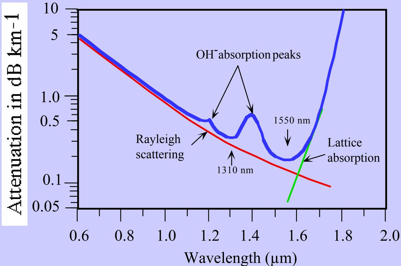
Illustration of a typical attenuation vs. wavelength characteristics of a silica based optical fiber. There are two communications channels at 1310 nm and 1550 nm.
