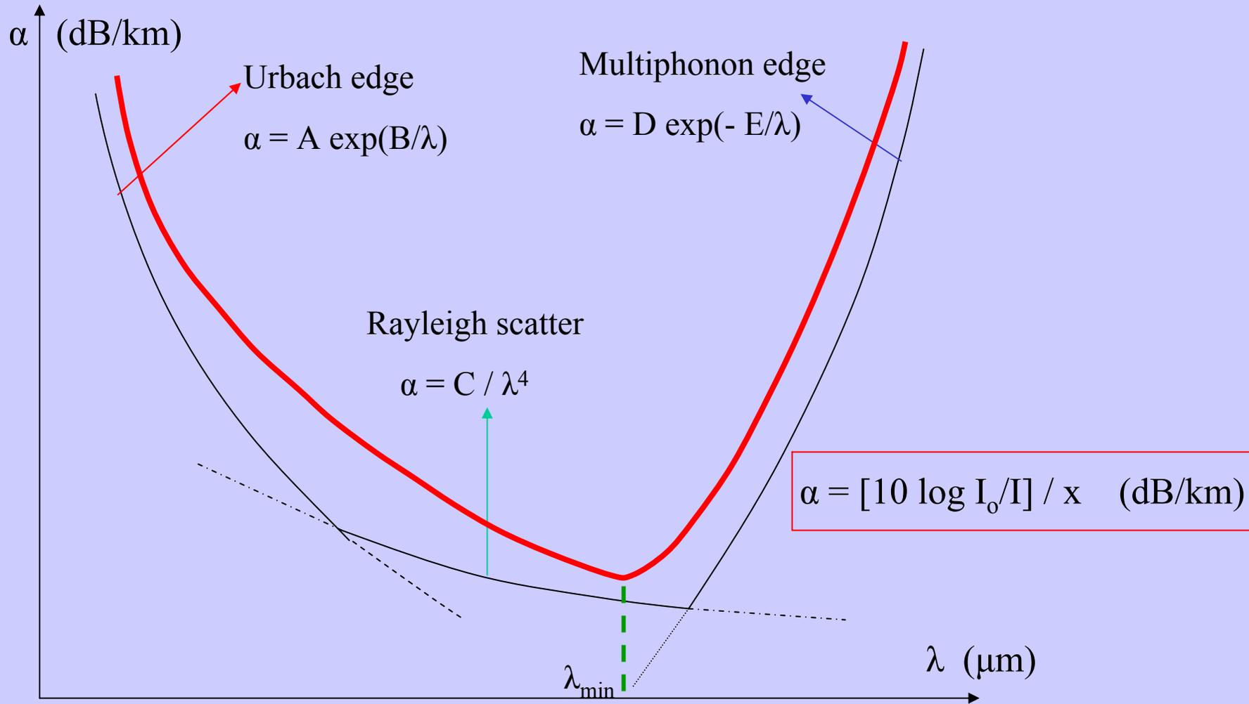
The wavelength of minimum loss,  $\lambda_{\min}$ , is usually located near the intersection of the Rayleigh scattering and multiphonon absorption curves.
