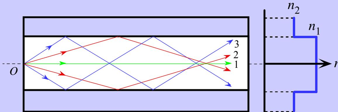
(a) Multimode step index fiber. Ray paths are different so that rays arrive at different times.
