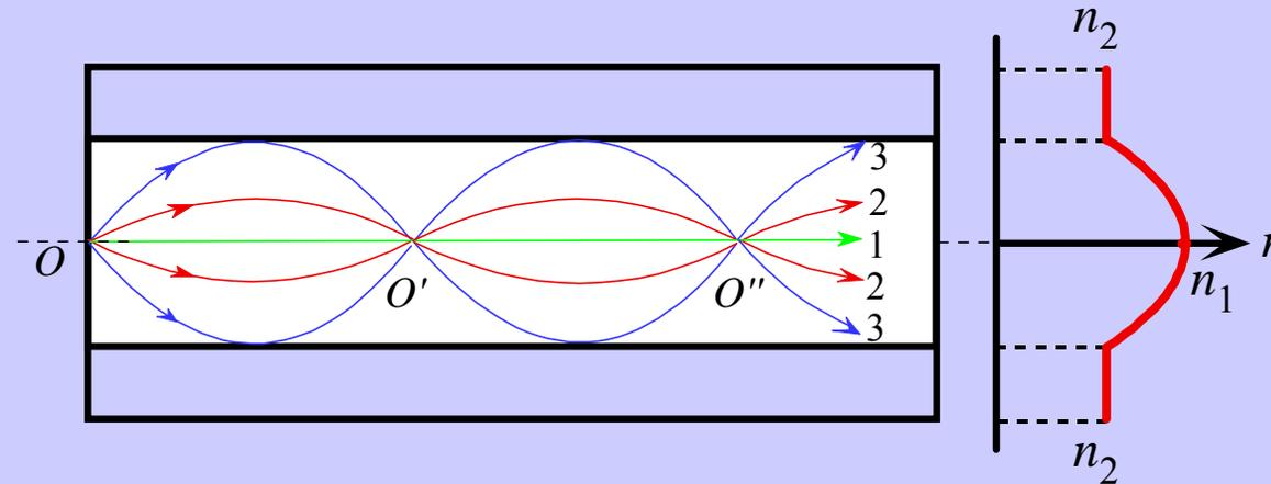
(b) Graded index fiber. Ray paths are different but so are the velocities along the paths so that all the rays arrive at the same time. (Strictly true for meridional rays).
