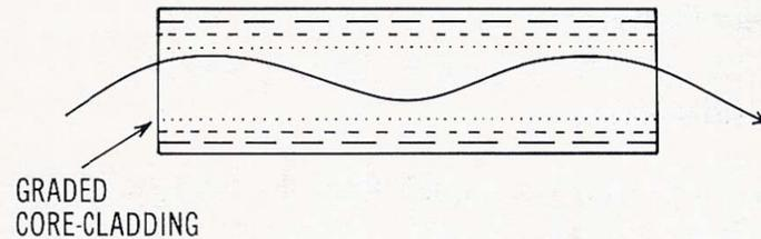
**A graded-index fiber.** Repeated focusing and refocusing.
