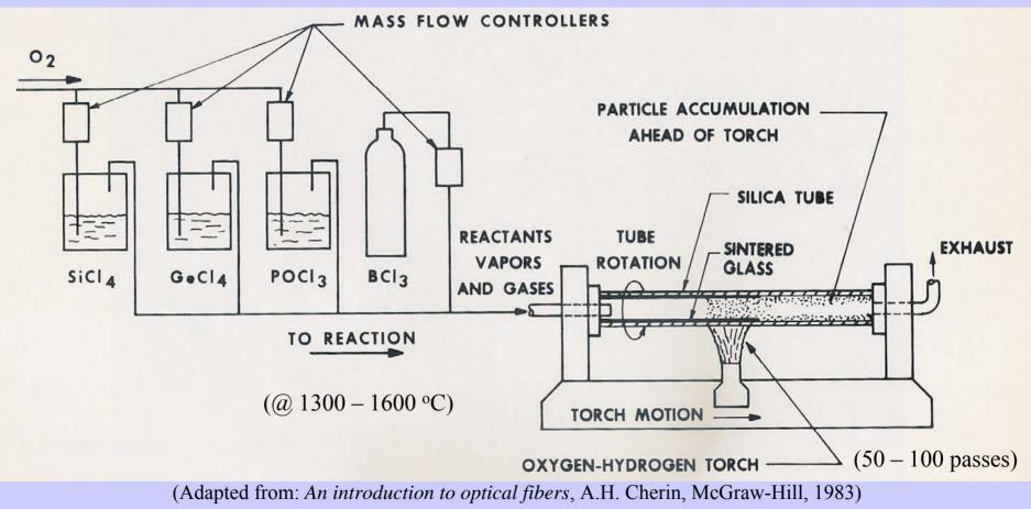
The final consolidation of the glass preform may be achieved with 4-5 passes of the torch  $@ \sim 1900 \text{ °C}.$
