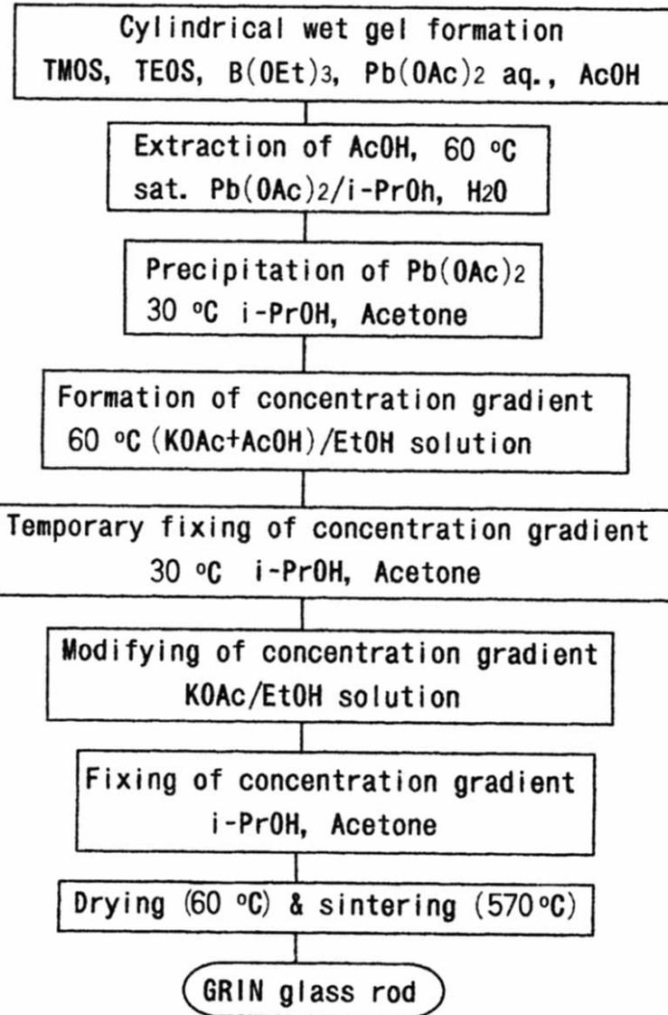
Fabricating process of GRIN rods by sol-gel process based on the interdiffusion of  $\text{Pb}^{2+}$  and  $\text{K}^{+}$  ions. [Reprinted from M. Yamane and S. Noda, *J. Ceram. Soc. Jpn.* **101** (1993) 11,
