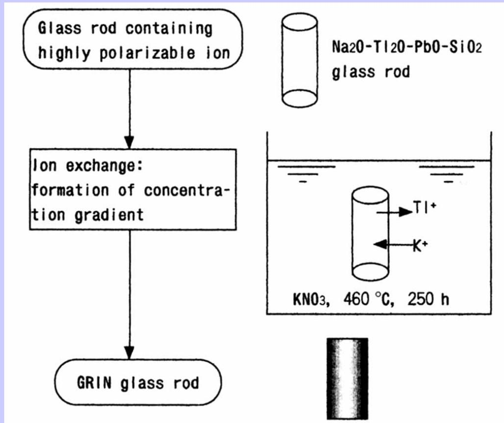
**Ion exchange process for fabricating r-GRIN rod.**
