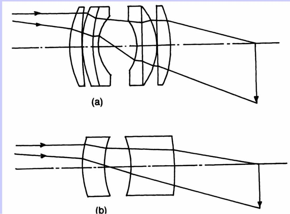
Configurations of (a) new double Gauss photographic objective, and (b) GRIN photographic objective. [Reprinted from L. G. Atkinson, S. N. Houde-Walter, D. T. Moore, D. P. Ryan and J. M. Stagaman, *Appl. Opt.* **21** (1982) 993, copyright (1982) with permission from the Optical Society of America.]
