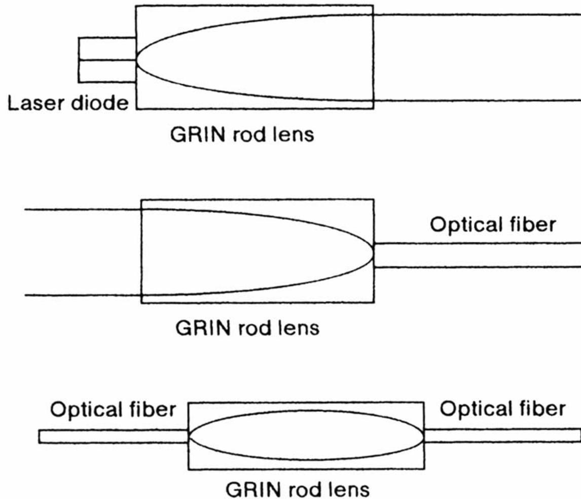
Schematic cross section of a coupler and collimator using GRIN rod lenses with small diameter and flat surface.
