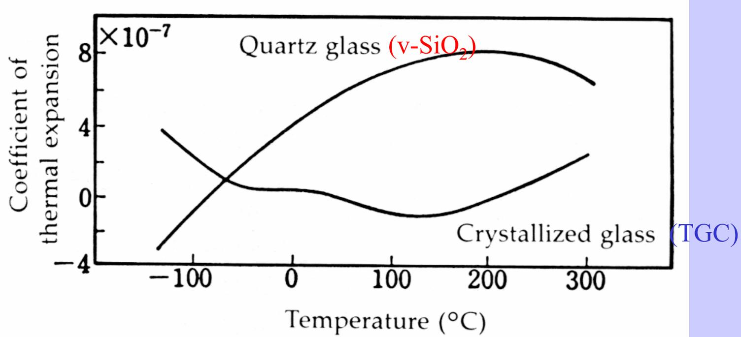
**Coefficients of thermal expansion of quartz glass and SiO<sub>2</sub>-Li<sub>2</sub>O-Al<sub>2</sub>O<sub>3</sub> crystallized glass.**
