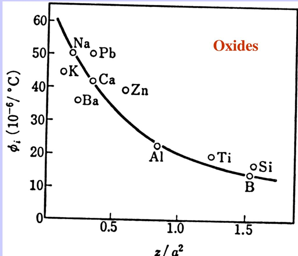
Relationship between cationic field strength ( $z/a^2$ ) and temperature coefficient of electron polarizability ( $\phi_i$ ) of ions.
