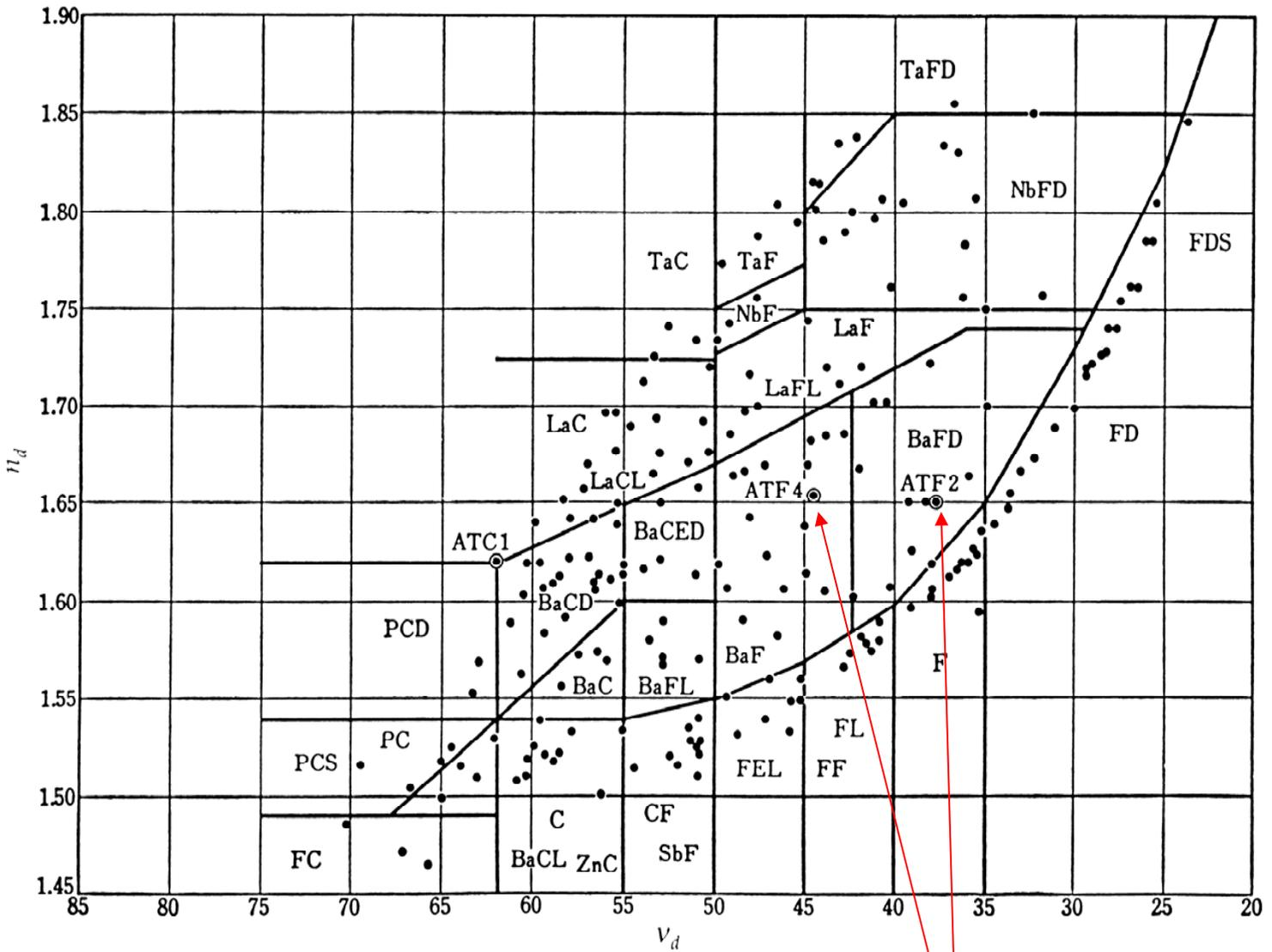
Graph of  $n_d - v_d$ . Glasses marked with  $\odot$  in the graph are athermal glasses.
