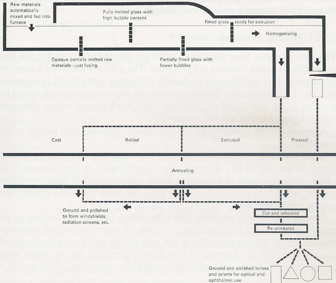
*The bubble free glass may be cast into blocks, rolled into sheets, extruded into bars, or pressed into blanks. After careful annealing it may be further processed by remoulding, grinding and polishing*
