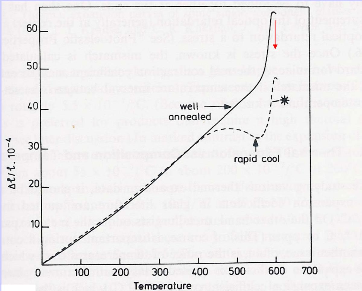
Effect of the initial cooling rate on the expansion of a glass.
