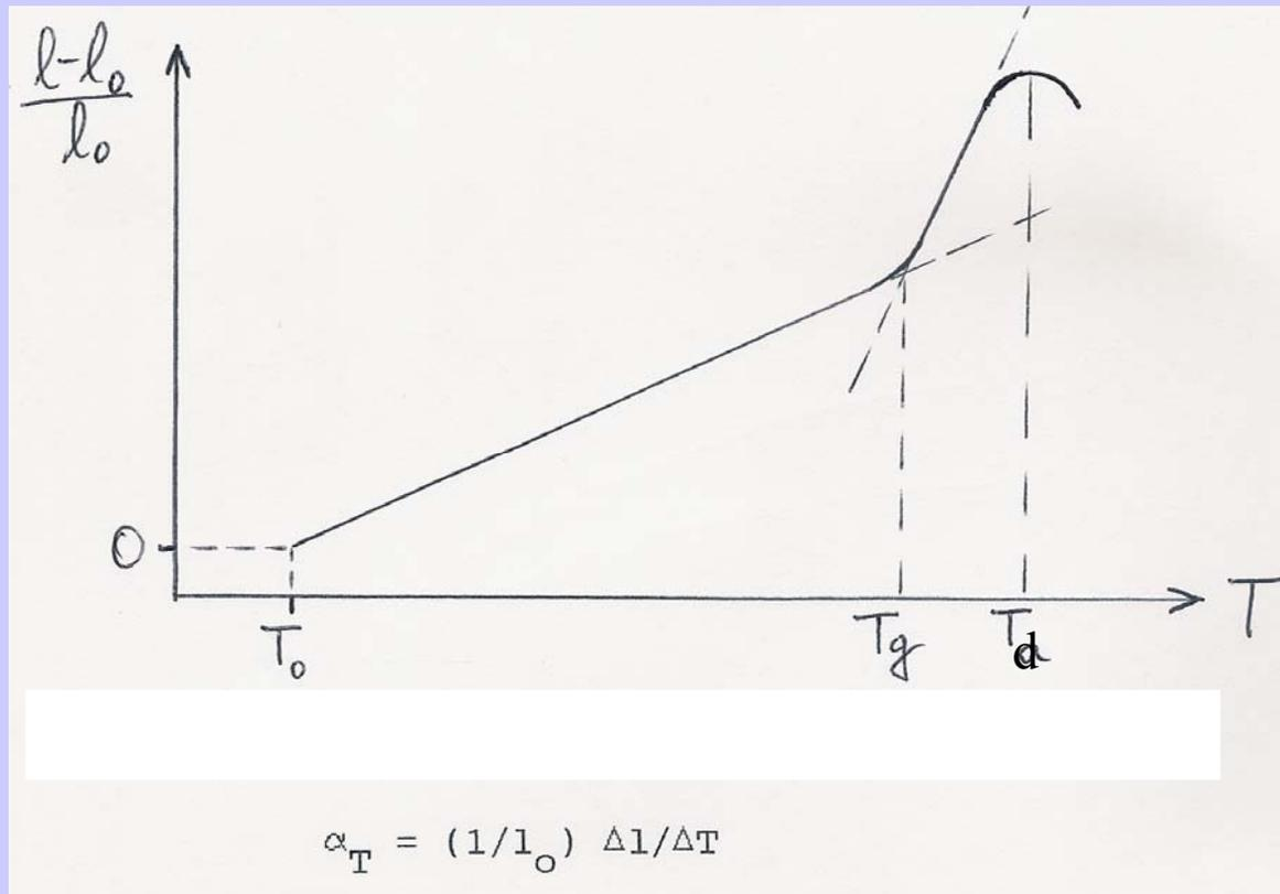
The curvature downwards is an artifact due to an apparent contraction caused by a pushrod penetration into the specimen, due to its softening. The rapidly cooled glass is less dense than the well annealed one and it will shrink, up to a certain point, when slowly reheated, as a result of structural relaxation.
