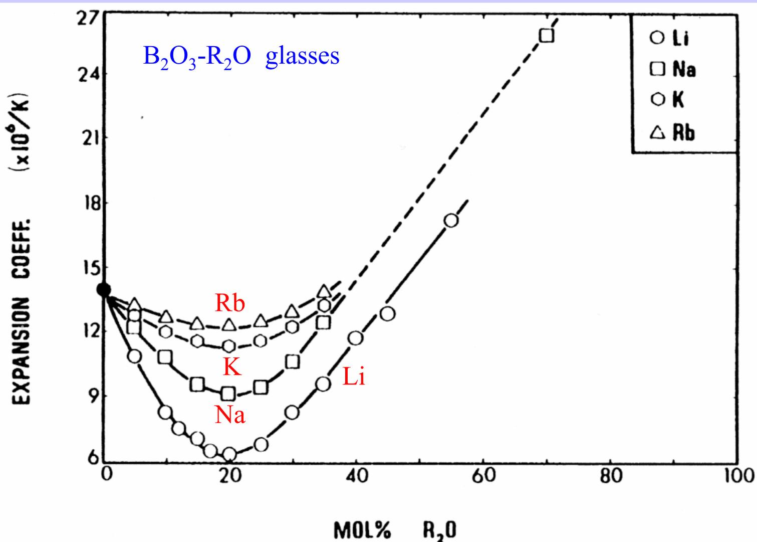
Thermal expansion coefficients of  $\text{R}_2\text{O} \cdot \text{B}_2\text{O}_3$  glasses as a function of composition. (After J. E. Shelby, *J. Am. Ceram. Soc.*, **66**(3), 225–227 (1983).)
