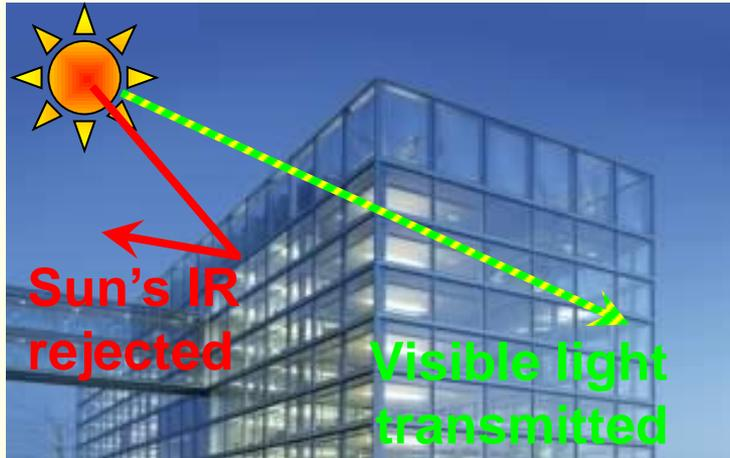
A **solar control** coating reflects near-UV and near-IR radiation from the sun, while transmitting the visible portion.
