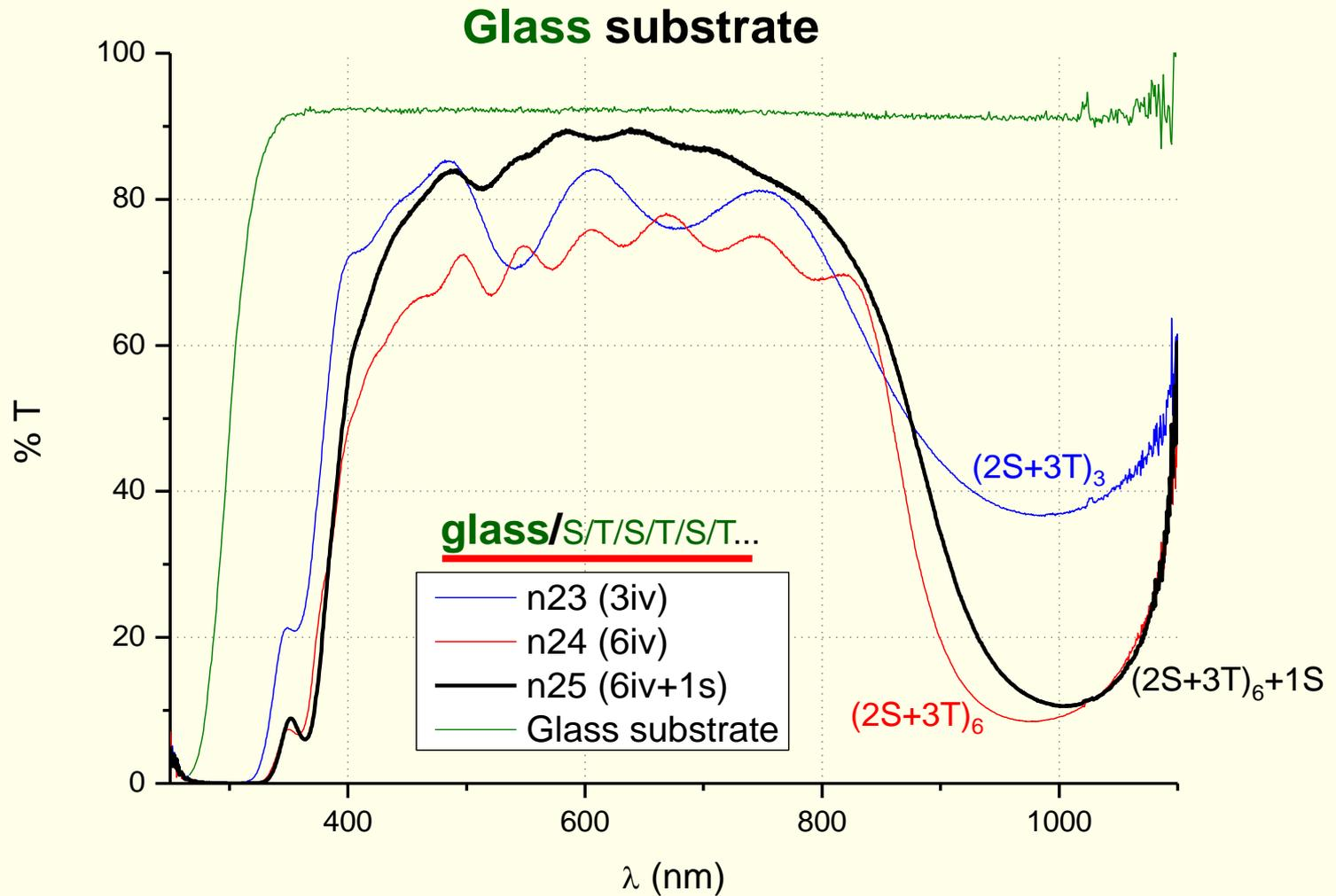
Nanostructured glass coatings for solar control
