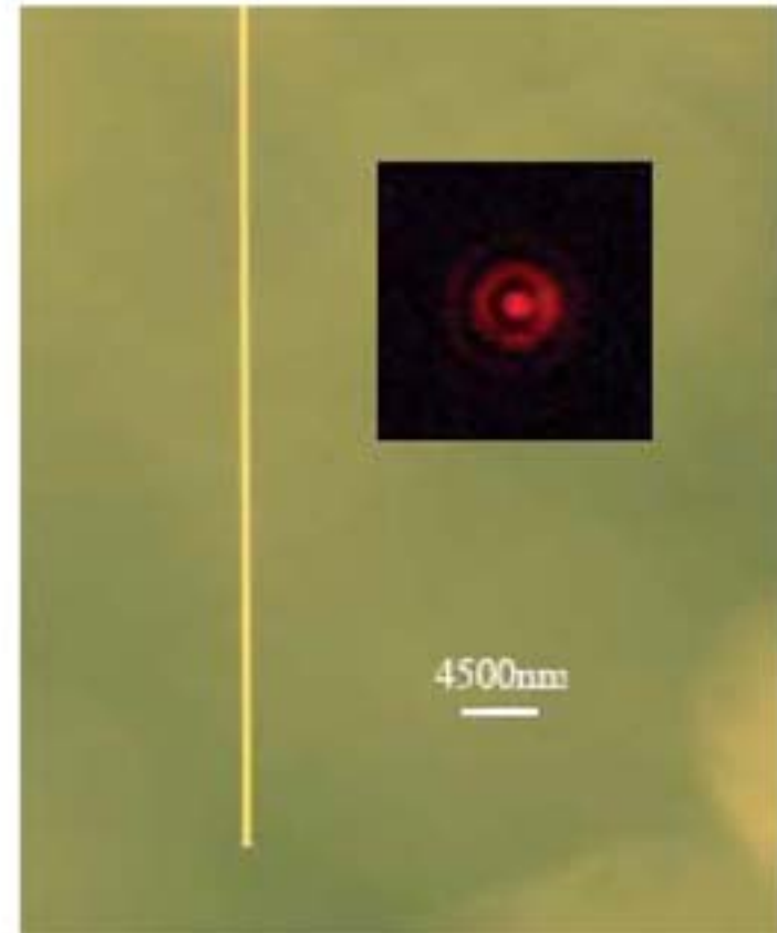
FIG. 1 (color online). The stationary micrograph of the tip of the SF, showing that the diameter of the SF tip is about 450 nm. The inset is the enlarged profile of a weak red light beam outgoing from the SF end face.
