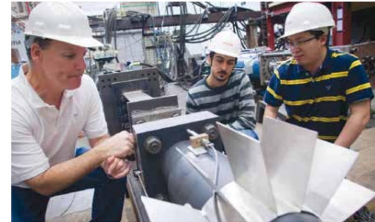
At the *NEES Lehigh Equipment Site*, Jim Ricles, left, and his graduate research assistants inspect a viscous damper after a laboratory seismic simulation. The researchers are developing performance-based design procedures for building dampers that reduce seismic damage and promote community resiliency to earthquakes.
