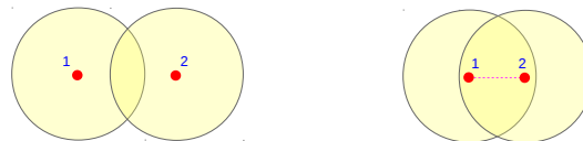
(a) Robots can't see each other, and hence have no way of detecting that their disks of visibility overlap. (b) Robots can see each other, and hence know that their disks of visibility overlap. Visibility is represented by the dotted magenta line.
