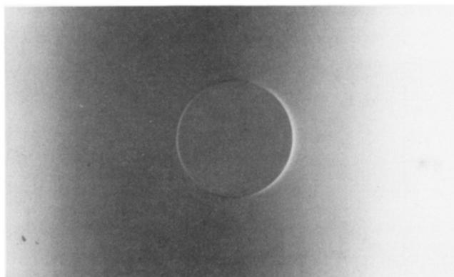
**Figure 3.** Photomicrograph showing the contact area (radius = 154  $\mu\text{m}$ ) resulting from the contact (in air) between a lens ( $R = 1.44 \text{ mm}$ ) and a flat sheet of PDMS. The edge of the lens is outside the field of view. There was no external load on the lens and hence the deformation was solely due to the effect of surface forces.
