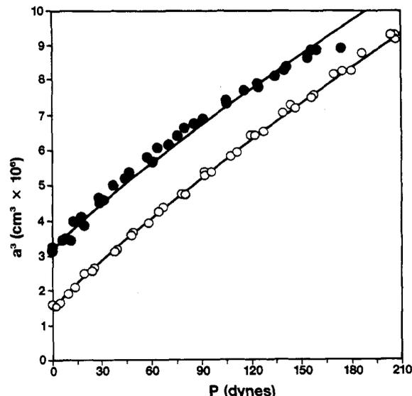
**Figure 15.** Results of the load-deformation experiments using a lens of PDMS<sup>0x</sup>-O<sub>3</sub>Si(CH<sub>2</sub>)<sub>9</sub>CH<sub>3</sub> and a flat sheet of PDMS<sup>0x</sup>-O<sub>3</sub>Si(CH<sub>2</sub>)<sub>2</sub>(CF<sub>2</sub>)<sub>7</sub>CF<sub>3</sub>. The open (O) symbols indicate the data obtained from increasing loads and the closed symbols (●) represent the data obtained from decreasing loads.
