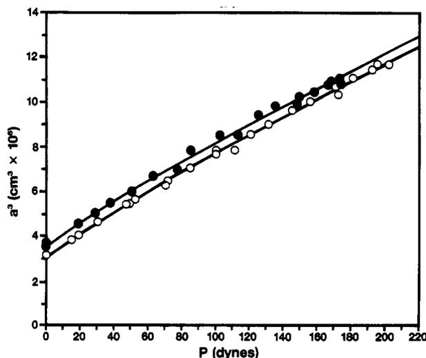
Figure 13. Plots of  $a^3$  against  $P$  showing weak hysteresis for the surfaces of  $\text{PDMS}^{\text{ox}}-\text{O}_3\text{Si}(\text{CH}_2)_9\text{CH}_3$ . The radius of the lens was 1.4 mm. The open circles (O) represent the data obtained from the increasing loads and the closed circles (●) represent the data obtained from the decreasing loads. The solid lines in both plots are predicted from eq 1.
