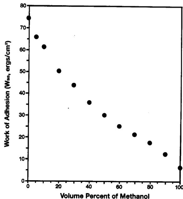
**Figure 7.** Works of adhesion ( $W_{sl}$ ) between two PDMS surfaces in mixtures of water and methanol plotted against the volume percent of methanol in the mixtures. To generate this plot, the data obtained from the deformation experiments under the mixtures of water and methanol were analyzed according to eq 4. The radius of the lens used in these experiments was  $1.52 \text{ mm}$ .
