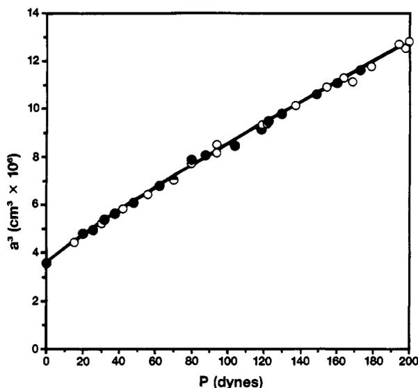
**Figure 4.** Plot of  $a^3$  against  $P$  following the form expected from eq 1. The data were obtained from the load-deformation experiments using unmodified PDMS. The radius of the lens used in these measurements was 1.44 mm. The open circles (O) represent the data obtained from increasing loads and the closed circles (●) represent the data obtained from decreasing loads: there is no hysteresis. The solid line was obtained from the analysis of these data by using eq 1.
