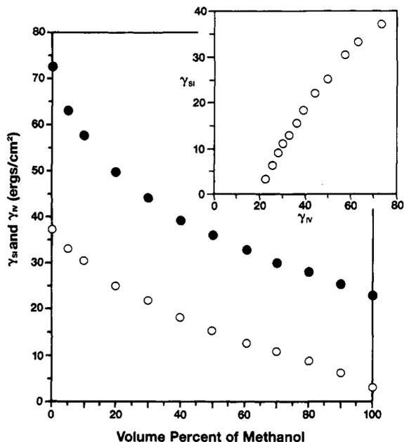
**Figure 8.** Surface tensions ( $\gamma_{lv}$ ) of water-methanol mixtures at the air-solution interfaces compared with the interfacial free energies ( $\gamma_{sl}$ ) of water-methanol mixtures at PDMS-liquid interfaces. The closed symbols (●) represent  $\gamma_{lv}$  and the open symbols (○) represent  $\gamma_{sl}$ . In the inset,  $\gamma_{sl}$  is plotted against  $\gamma_{sv}$ .
