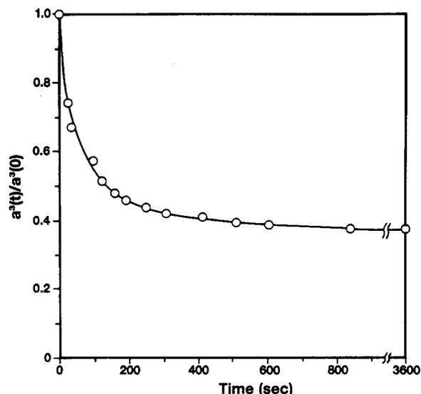
**Figure 16.** Area of contact between a lens of PDMS<sup>ox</sup>-O<sub>3</sub>Si-(CH<sub>2</sub>)<sub>9</sub>CH<sub>3</sub> and a flat sheet of PDMS<sup>ox</sup>-O<sub>3</sub>Si(CH<sub>2</sub>)<sub>2</sub>(CF<sub>2</sub>)<sub>7</sub>CF<sub>3</sub> as a function of time when a load is applied on the lens and then removed. The data are presented in the dimensionless form,  $a^3(t)/a^3(0)$ , where  $a(t)$  is the contact radius at time  $t$  and  $a(0)$  is the initial contact radius.
