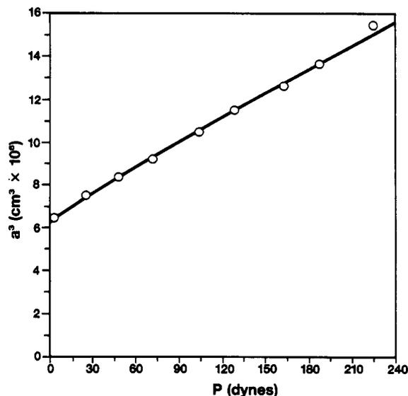
Figure 12. Plot of  $a^3$  against  $P$  for  $\text{PDMS}^{\text{ox}}$  following the form expected from eq 1. The data were obtained from the loading experiments only. The radius of the lens was 1.21 mm.
