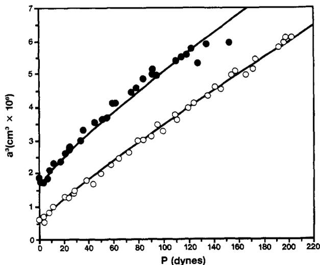
**Figure 14.** Plots of  $a^2$  against  $P$  for the surfaces of PDMS<sup>0x</sup>-O<sub>3</sub>Si(CH<sub>2</sub>)<sub>2</sub>(CF<sub>2</sub>)<sub>7</sub>CF<sub>3</sub> exhibiting large hysteresis. The radius of the lens was 1 mm. The open circles (O) represent the data obtained from the increasing loads and the closed circles (●) represent the data obtained from the decreasing loads. The solid lines are obtained from the analysis of these data using eq 1.
