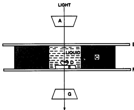
**Figure 6.** Contact deformations under liquids measured by placing a lens (D) in contact with a flat sheet (E) of PDMS in a liquid medium. The experimental cell is made of Sylgard 170 (C), which has a rectangular hole at the center. The cell is sandwiched between two glass slides (B and F). This assembly is placed in between the condenser (A) and objective (G) of an optical microscope.
