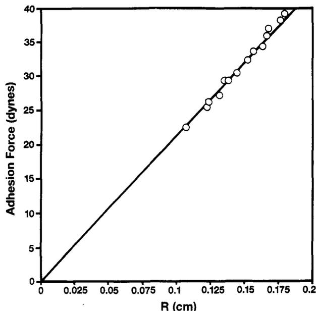
**Figure 11.** Adhesion (pull-off) forces between semispherical lenses and a flat sheet of PDMS varying linearly with the radius ( $R$ ) of curvature of the lenses. These data are in accordance with eq 13. The surface free energy of PDMS obtained from this plot is 22.6 ergs/cm<sup>2</sup>.
