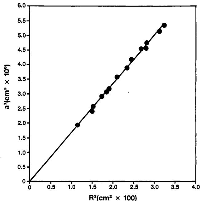
**Figure 5.** Plot of  $a^3$  against  $R^2$  following eq 4. The data were obtained from the contact deformations of lenses of various sizes and a flat sheet of PDMS in air. There was no external load on these lenses, and thus the deformations were purely due to surface forces.
