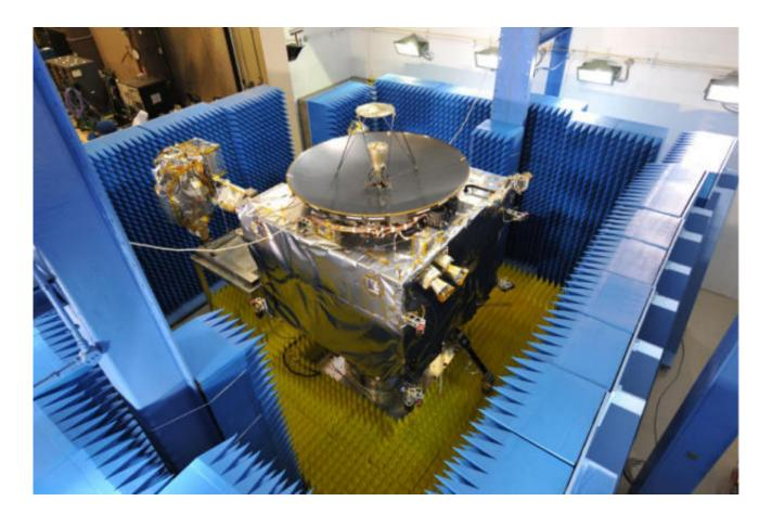
The MAVEN spacecraft, during electromagnetic interference/electromagnetic compatibility testing. (Credit: Lockheed Martin) Unless the Mars Curiosity rover has, unbeknownst to us, been writing poetry in addition to **singing "Happy Birthday" to itself [http://www.cnet.com/8301-17938 105-57597122-1/mars-curiosity-rover-sings-happy-birthday-toitself/]**, haiku has yet to reach the fourth rock from the sun.
