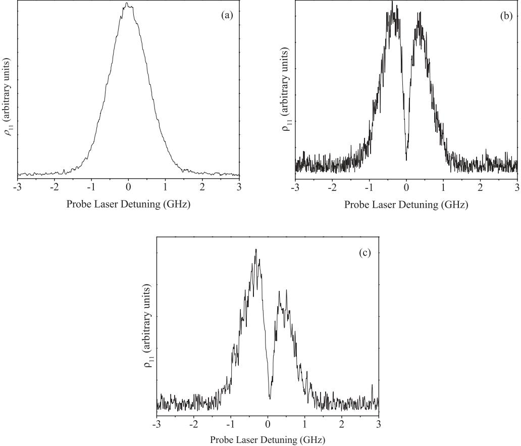
FIG. 3. Experimental spectra for  $\text{Na}_2$  V-system probe laser scans in the copropagating geometry (a) with the coupling field turned off and (b) with the coupling field on and the frequency of the coupling laser set to line center of the transition. (c) The coupling field is detuned by  $\sim 60$  MHz. The coupling laser power is 265–270 mW and the probe laser power is less than 1 mW.
