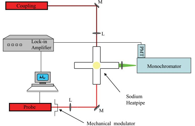
FIG. 2. (Color online) Experimental setup for the V-scheme EIT experiment. The coupling and probe laser beams propagate in opposite directions. A mechanical chopper is used to modulate the probe field while neutral density filters allow the attenuation of each laser field. M = mirror, L = lens.
