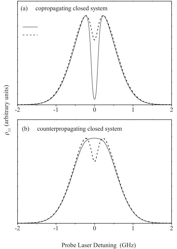
FIG. 11. Comparison between (a) co- and (b) counterpropagating fluorescence signals for the cases of  $\rho_{13} \neq 0$  (solid line) and  $\rho_{13} = 0$  (dashed line) in a closed 3-level V-type system. The calculation of the population of level  $|1\rangle$  is carried out using parameters close to the experimental conditions:  $\Omega_1/(2\pi) = 10$  MHz,  $\Omega_2/(2\pi) = 220$  MHz,  $\gamma_{ij}^{\text{col}}/(2\pi) = 0.79$  MHz.
