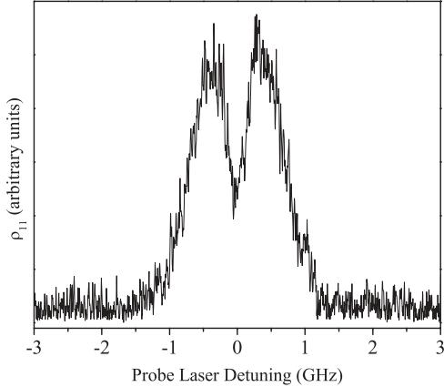
FIG. 4. Experimental spectra for counterpropagating laser beams. While the coupling field is on resonance, the probe field is scanned and fluorescence from level  $|1\rangle$  (which is proportional to the level  $|1\rangle$  population) is recorded. The powers of the coupling and probe lasers were 350 mW and 120  $\mu$ W, respectively.
