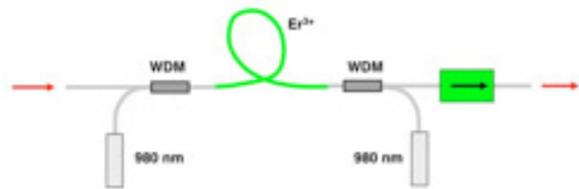
Fig. 4. (a) Basic set-up of a EDFA
