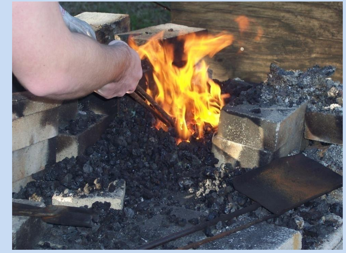
Fig. 3 – Heating the material in preparation for forging a knife blade.
