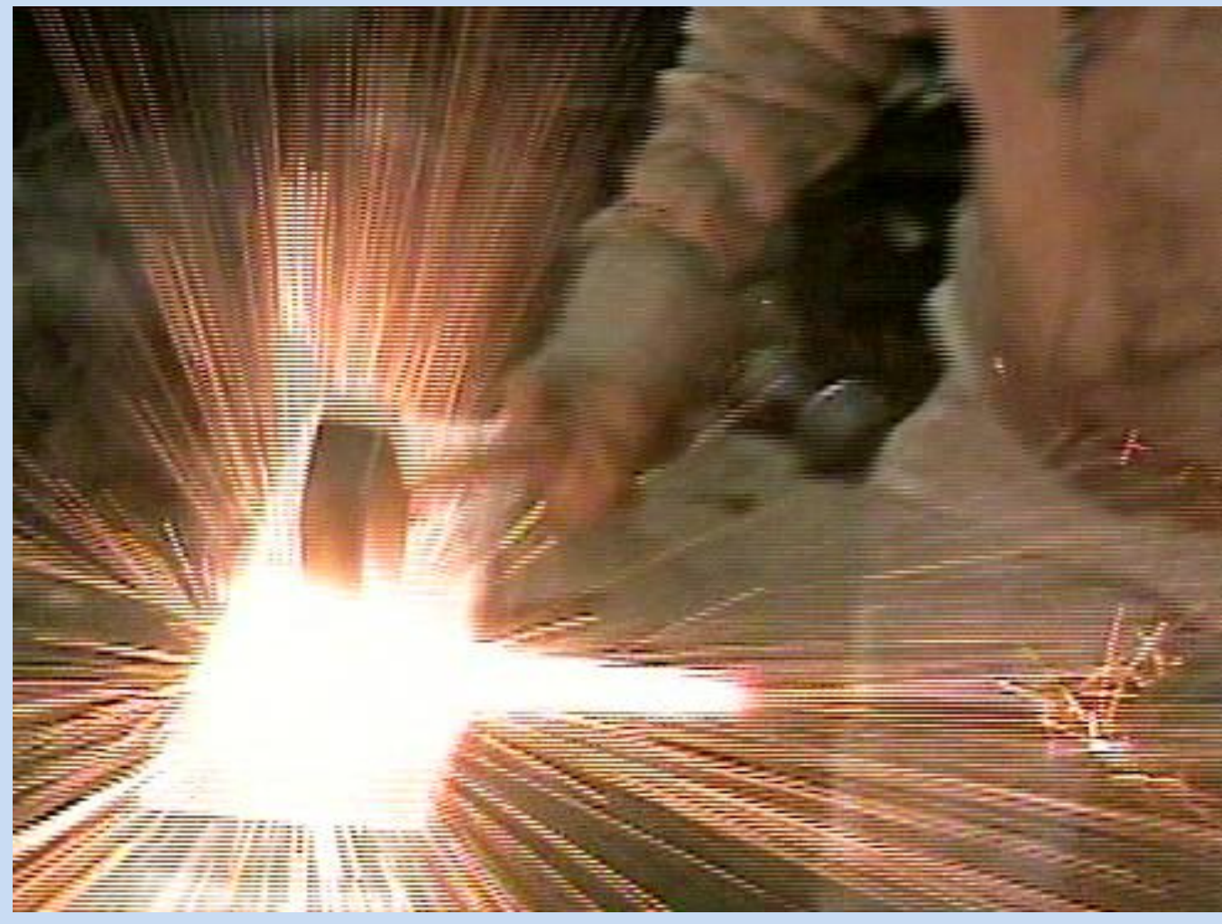
Fig. 1 – Forge-welding the layers together.
