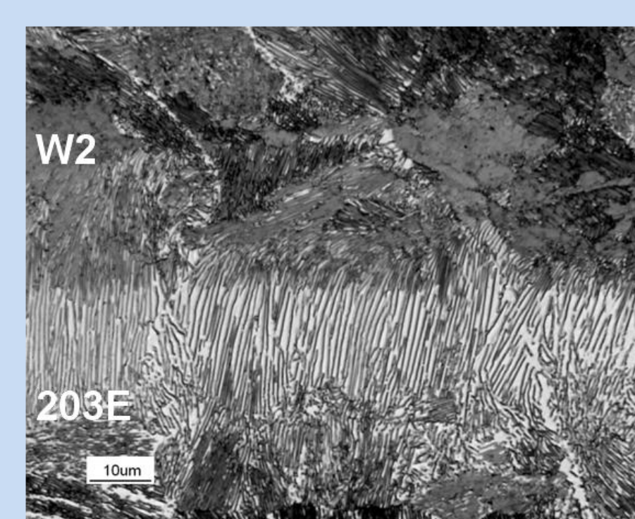
Fig. 11 – Interface in 256 layer sample. Etched in 4% picral.
