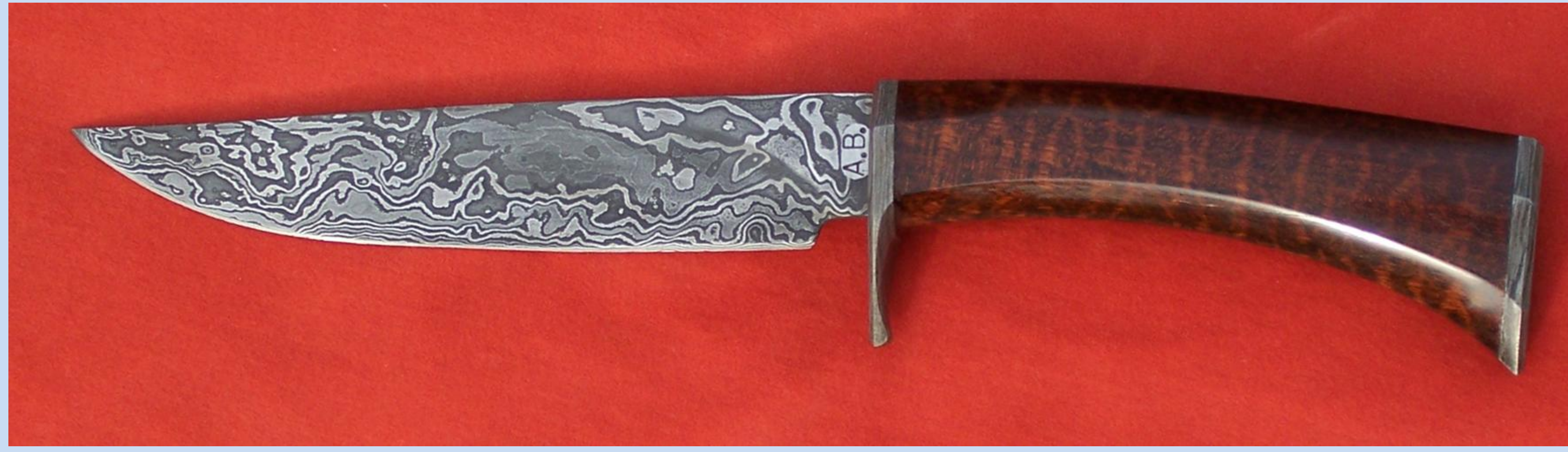
Fig. 2 – An example of a finished pattern-welded steel knife etched with 12% FeCl 3 . Forged by the author.
