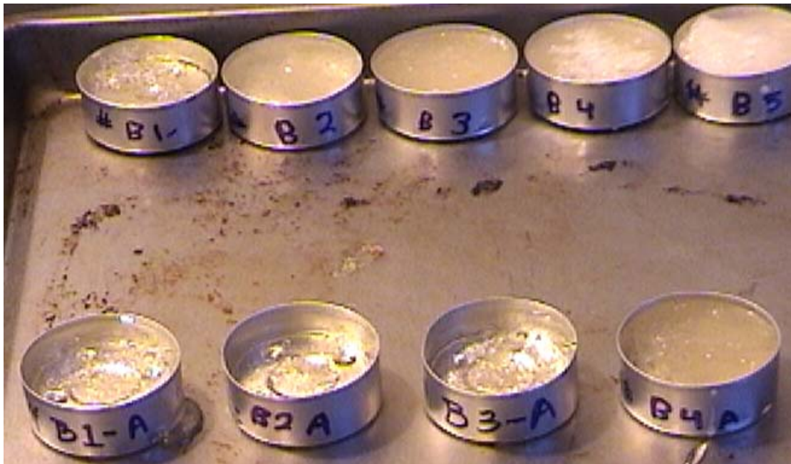
Fig. 3. The figure shows the effect of melt-stirring on glass formation. The samples in top row were stirred before casting, whereas the ones on bottom row were not stirred.
