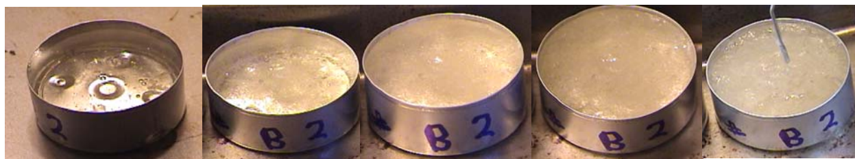
Fig. 4. Growth of sugar crystals in high modifier content mixture. The figure shows B2 sample with increasing time from left to right.
