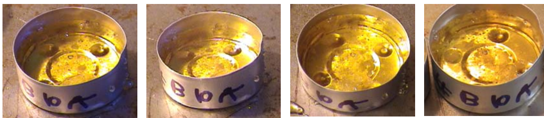
Fig. 4. Growth of sugar crystals in high modifier content mixture. The figure shows B2 sample with increasing time from left to right.
