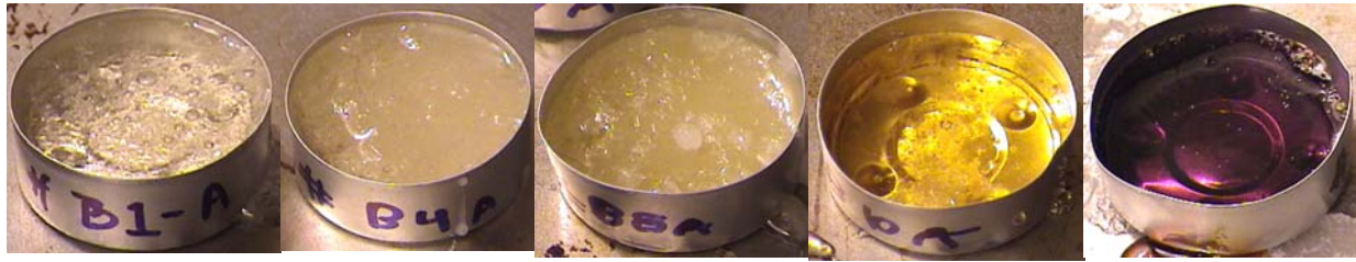
Fig. 6. Demonstration of increasing glass-forming ability with decreasing modifier content from left to right. Unstirred sugar+H 2 O samples from Experiment B(a). Sample #B1(a) is mostly liquid with a few crystals floating. The fraction of crystals increases in #B4(a) and #B8(a), the latter being mostly solid. #10(a) is mostly solid glass with a few crystalline regions. Finally, the last sample (#B12(a)) is just solid glass.
