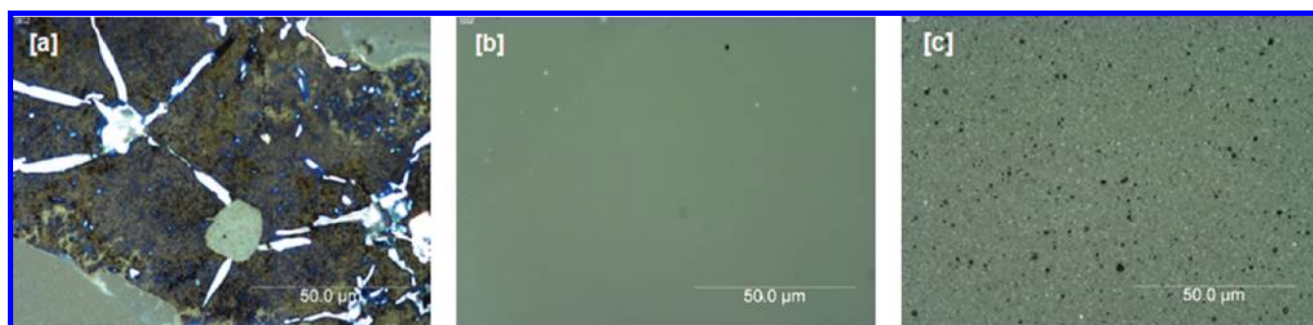
FIGURE 7. Optical micrographs of the glass surfaces exposed to 85 °C and 85% relative humidity for 10 days: (a) pristine float glass; (b) carbon-coated float glass made using PR (10:1) as the precursor; (c) carbon-coated float glass made using a 0.5 wt % CTP solution as the precursor.
