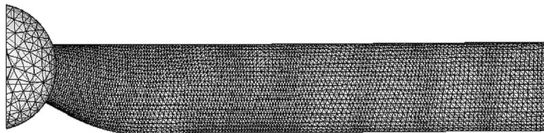
FIG. 3. Finite element mesh used for structural solver.
