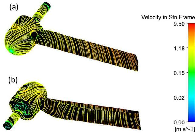
FIG. 13. Streamlines of velocity in stationary reference frame on (a) upwind side and (b) downwind side of the turbine blade.
