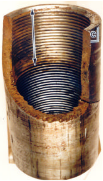
Photograph of a failed shaft coupling from a vertical circulator water river pump that operated at a nuclear power station.
