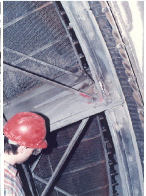
(b) ERC researcher conducts field evaluation of air preheater cold end fouling.
