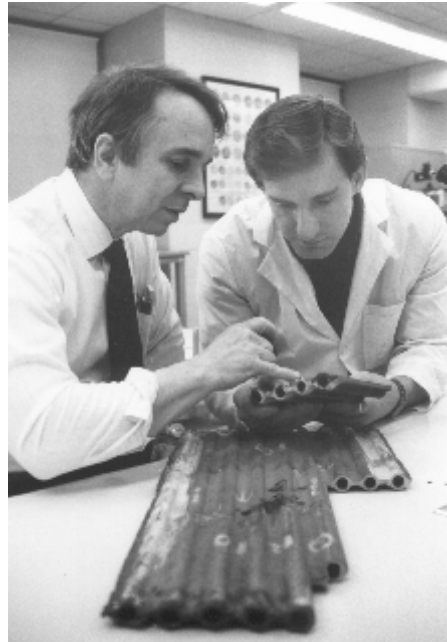
(a) Research Scientist Arlan Bescoter (left) examines a failed boiler tube for an Energy Liaison Program member company.
