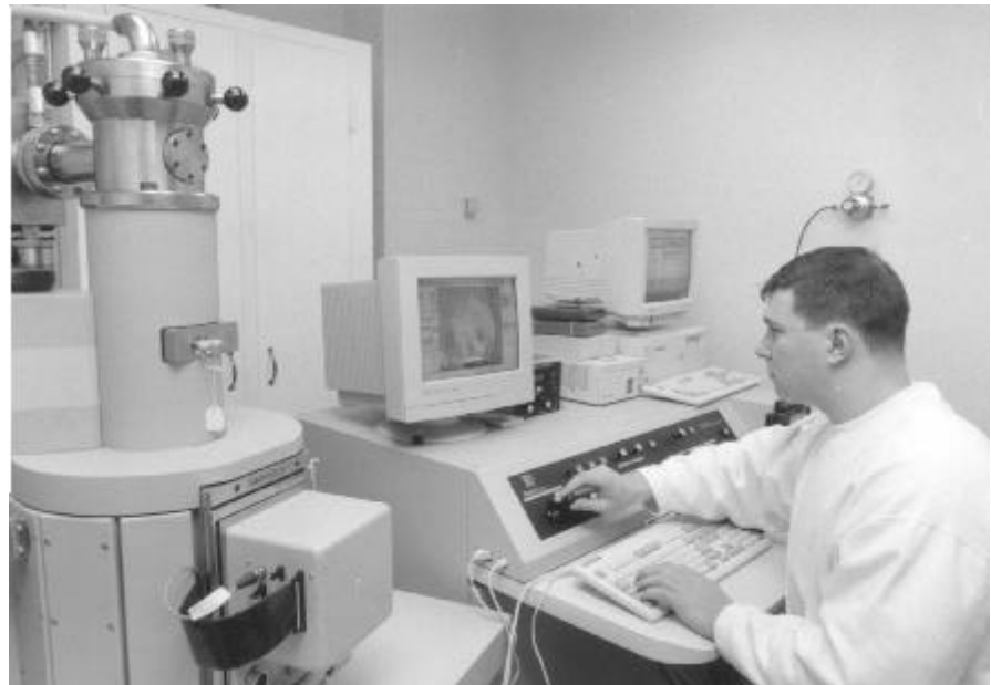
Graduate student Steve Banovic is using a Environmental Scanning Electron Microscope to examine the microstructure of an electrodeposited coating.
