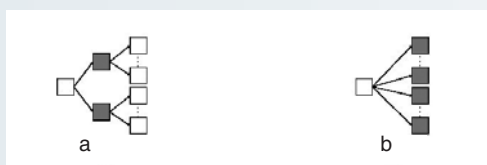
Figure 3: (a) Hub-and-spoke network and (b) point-to-point network. The sites that hold inventory are shaded.
