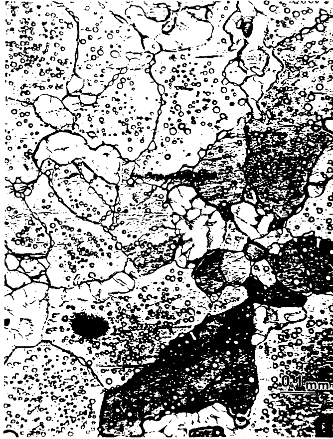
Fig.17. Optical micrograph of large grain size of copper matrix after etching (x 100)
