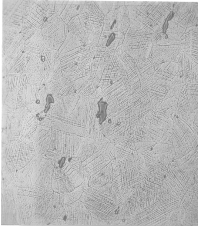
Fig.18. SEM micrograph of tin-bronze axe (x720). Cordiform implement (T5126)
