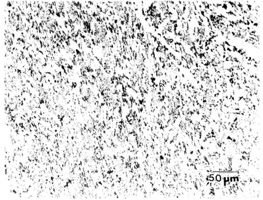
FIG. 8. *Denarius* of Faustina, ~22wt.% Cu, ferric chloride etch.
