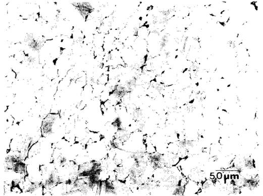
FIG. 12. Core of coin of Aurelian; ferric chloride etch.
