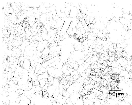
FIG. 3. *Denarius* of M. Tullia; single phase, <9wt.%Cu,  $K_2Cr_2O_7-H_2SO_4$  etch.
