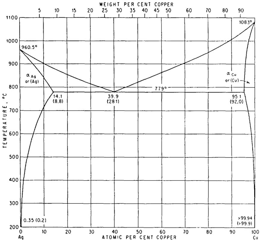
Fig. 2. The copper-silver phase diagram.
