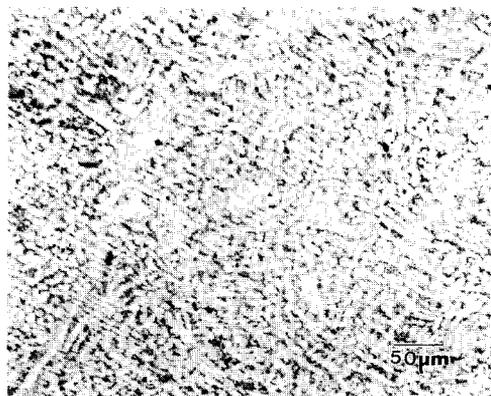
FIG. 5. *Denarius* of Titus; ~12 wt.%Cu, ferric chloride etch.
