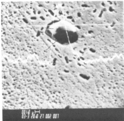
FIG. 3.--Axehead from Safadi-Abu Matar. Secondary-electron image (SEM) of inclusion with Ni Ka linescan superimposed.
