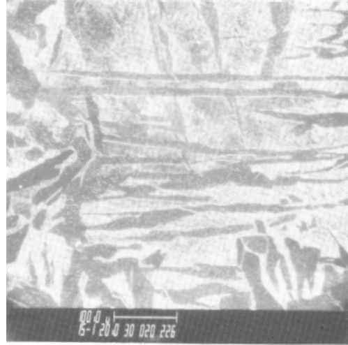
FIG. 2.--SEM image showing Widmanstatten ferrite.
