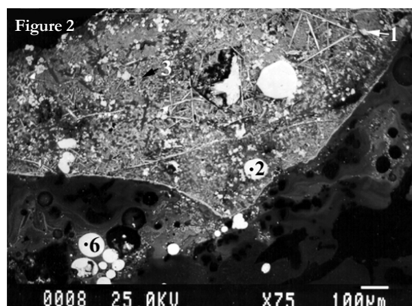
Figure 1 and 2: (fig 1) Sample M-F-05 is a typical furnace slag fragment showing skeletal fayalite (3) with intergrowth of magnetite (2) and some copper prills (1). (fig 2) EPMA micrograph of sample Miftan 1 showing the angular inclusion of smelting slag embedded in the glassy remelting slag. The data are presented in Table 1.
