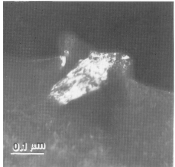
FIG. 8.--Dark-field image (TEM) of star-shaped precipitates.
