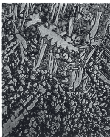
75-22-3 alpha plus (alpha and delta) (actually 22.7% tin)
