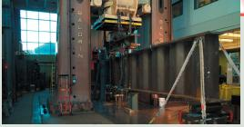
**NEES:** as part of the NSF-NEES Network allows for **R**eal-**T**ime **M**ulti-**D**irectional (RTMD) seismic testing, combined with real-time analytical simulations, to investigate the seismic behavior of large-scale structural systems.
