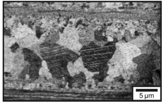
Fig. 4. Multiple layered vein showing bi-directional growth of calcite off seed nuclei on the vein walls inward toward the center where crystals enlarge. A few of the larger calcite crystals exhibit mechanical twin lamellae.
