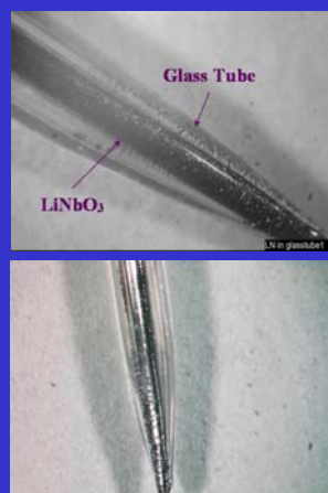
Single Crystal Fiber Encapsulation with Glass Capillary
