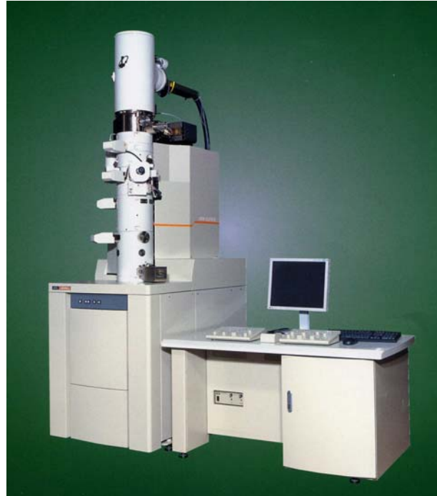
JEM 2200FS TEM with energy filter and CEOS aberration corrector
