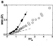
**Fig. 12.** (A) Variations of  $\langle r^2 \rangle$ , in the prediffusion regime with temperature for computer-simulated  $\mathrm{SiO_2}$  (3D network),  $\mathrm{B_2O_3}$  (2D sheet), and BOF (linear chains).  $T_{\rm g}$  values are given in parentheses. Included are laboratory neutron scattering data from (137) for the case of selenium, which has  $T_{\rm g}$ close to that of BOF. (B) Same data versus  $T/T_{o}$ where  $T_{a}$  is the calorimetric  $T_{a}$ .
