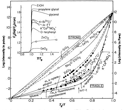
**Fig. 4.** Arrhenius plots of the viscosity data scaled by values of  $T_{\rm g}$  from Fig. 3 and other sources showing the "strong-fragile" pattern of liquid behavior on which the liquid's classification of the same name is based. As shown in the insert, the jump in  $C_{\rm p}$  at  $T_{\rm g}$  is generally large for the fragile liquids and small for strong liquids, although there are a number of exceptions, particularly when hydrogen bonding is present. [From (36)]
