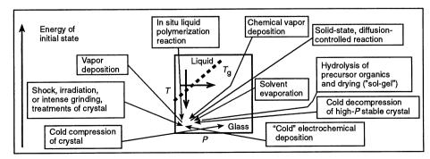
**Fig. 1.** Various routes to the glassy state, roughly indicating the energies of the initial states relative to the final glassy states. The route of crystal compression below  $T_{\rm g}$  may yield glasses that are thermodynamically distinct from those obtained by the other routes but which may transform to them by way of nonequilibrium first-order transitions.
