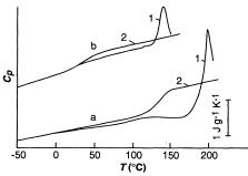
**Fig. 9.** Differential scanning calorimeter scans of the globular protein legumin both before and after denaturation, for different water contents (**A**) dry and (**B**) 10.4% by weight. Note the increase in calorimetric strengths of glass transitions after denaturation. The native state acts like a strong liquid. Comparison of the glass transition with a simple homopolypeptide, poly-L-asparagine is made in Fig. 10. [From (117b) by permission copyright Oxford University Press]
