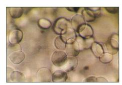
**Fig. 5.** Microstructure showing two glassy phases of identical composition formed by quenching an initially homogeneous oxide melt in the system  $Y_2O_3$ -Al $_2O_3$ . The droplet phase has a lower density and has evidently nucleated from the denser phase, which is a fragile liquid at 2000 K (Fig. 4), during quenching. [From (70) by permission copyright Macmillan]
