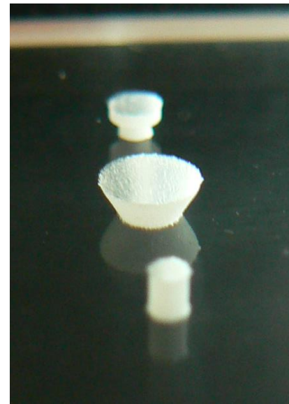
1mm drilling (straight, conical and counterbore)
