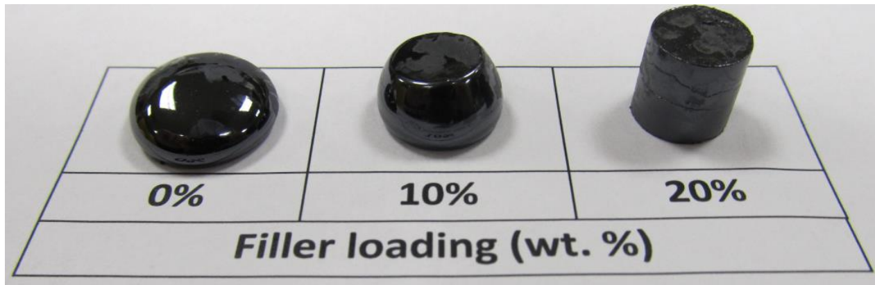
V-phosphate frit with different filler loadings fired at 380°-1h
