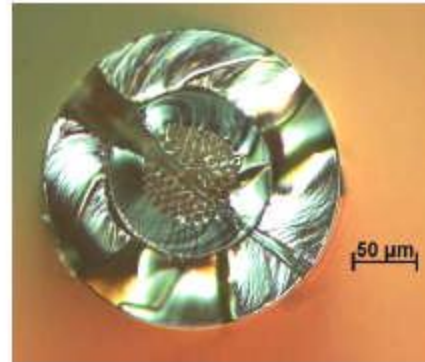
laser drilled PCF (cross section)
