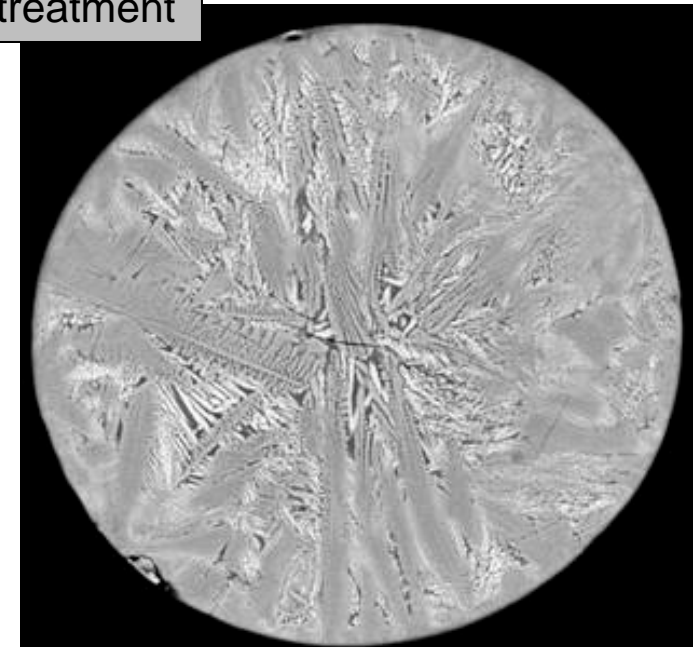
Fiber cross sections after heat treatment
